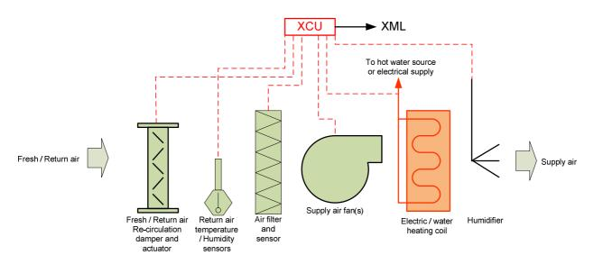
Figure 1: Air conditioning system (without chillers)
