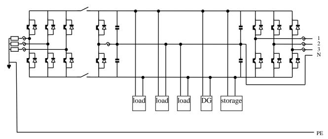
Figure 2: Example for a transfer static switch circuital schemes
