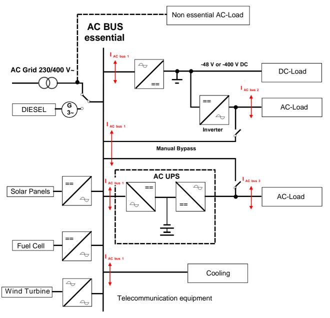
NOTE: The Network operator decides the structure, which equipment is to be connected to the essential (generator backed) (for instance fans of the cooling system) or non-essential AC distribution.
