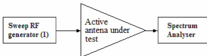
NOTE: The swept frequency range of the RF generator shall be greater than the nominal band of the active antenna as declared by the manufacturer.
