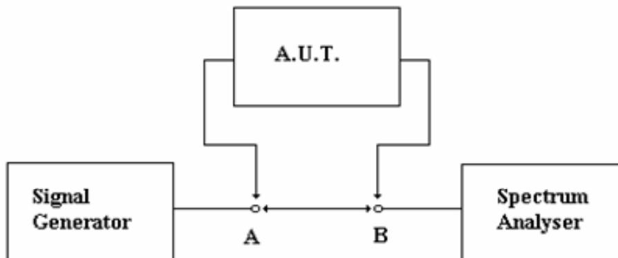
Figure 1: Measurement arrangement
