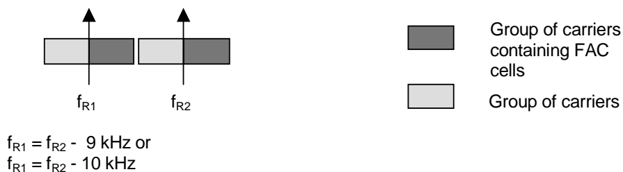
Figure K.6: Example of base/enhancement DRM signals
