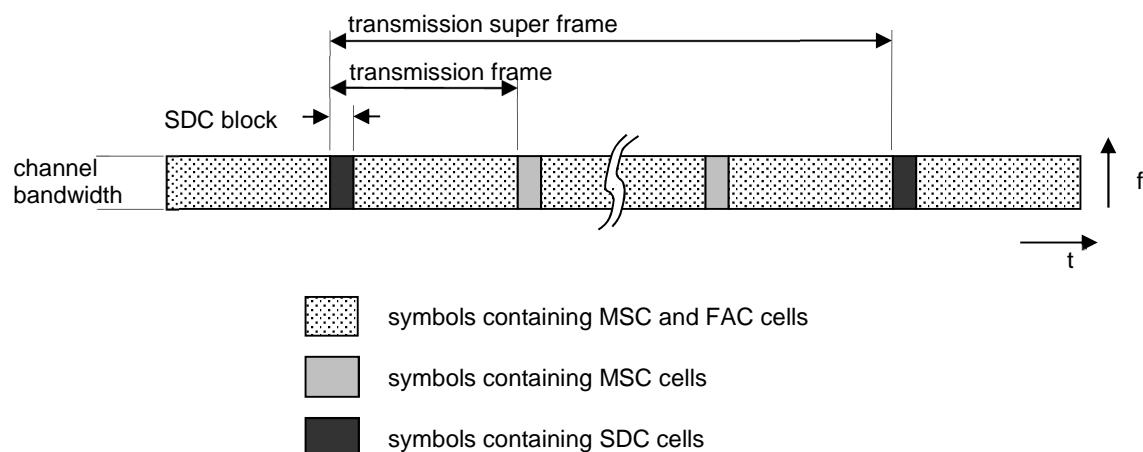
Figure 33: Time-frequency location of FAC and SDC signals
