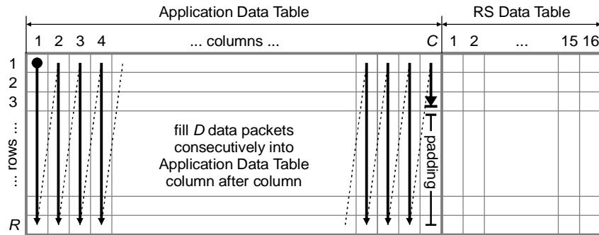
**Figure 14: Placing data packets into FEC frame**
