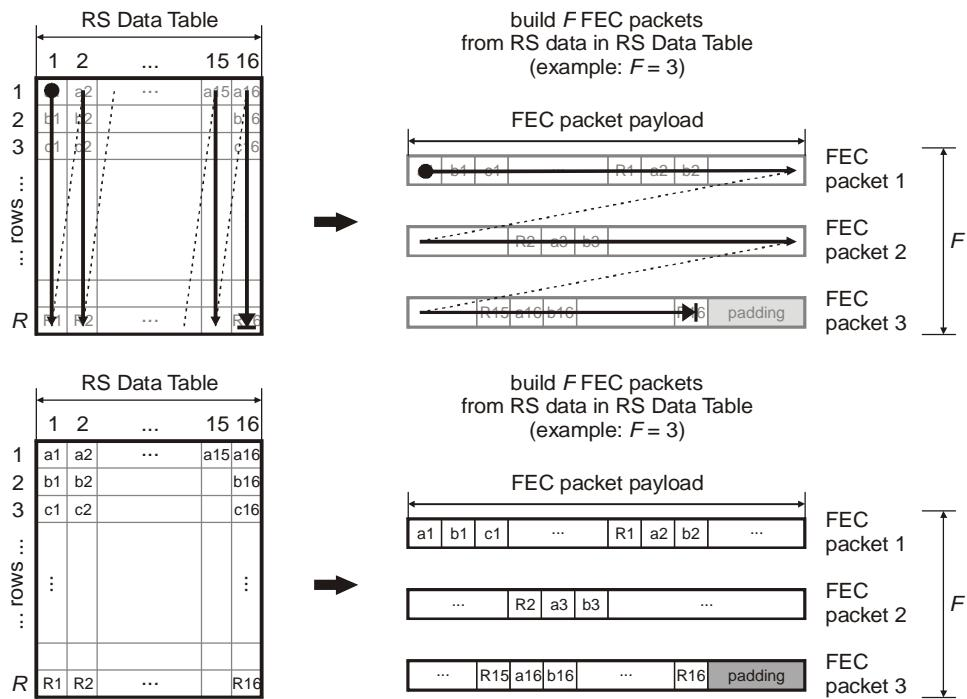
**Figure 16: RS data byte order within FEC packets**
