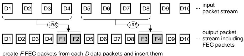
**Figure 17: Inserting FEC packets into the packet stream**
