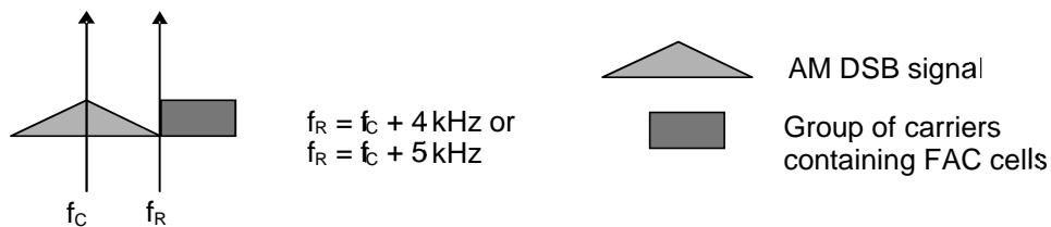
**Figure K.3: Example simulcast modes for half channel offsets**
