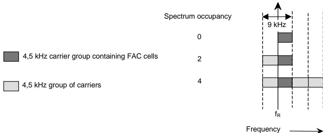
**Figure 31: Spectrum occupancy for 9 kHz channels**
