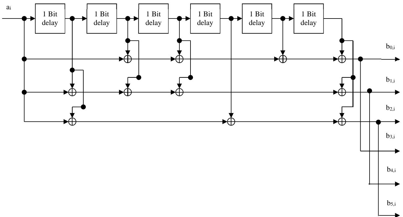
**Figure 25: Convolutional encoder**
