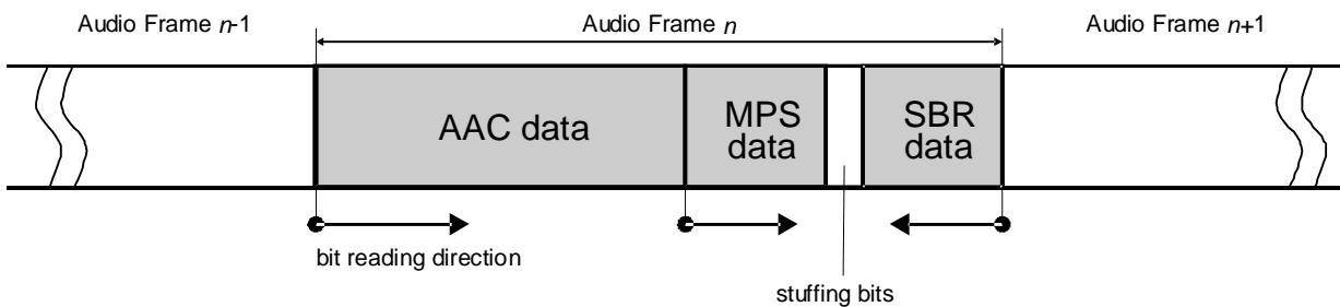
**Figure 11: AAC + SBR + MPS frame**
