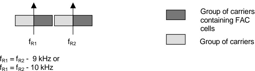
**Figure K.6: Example of base/enhancement DRM signals**
