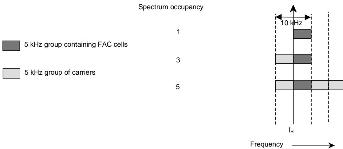
**Figure 32: Spectrum occupancy for 10 kHz channels**
