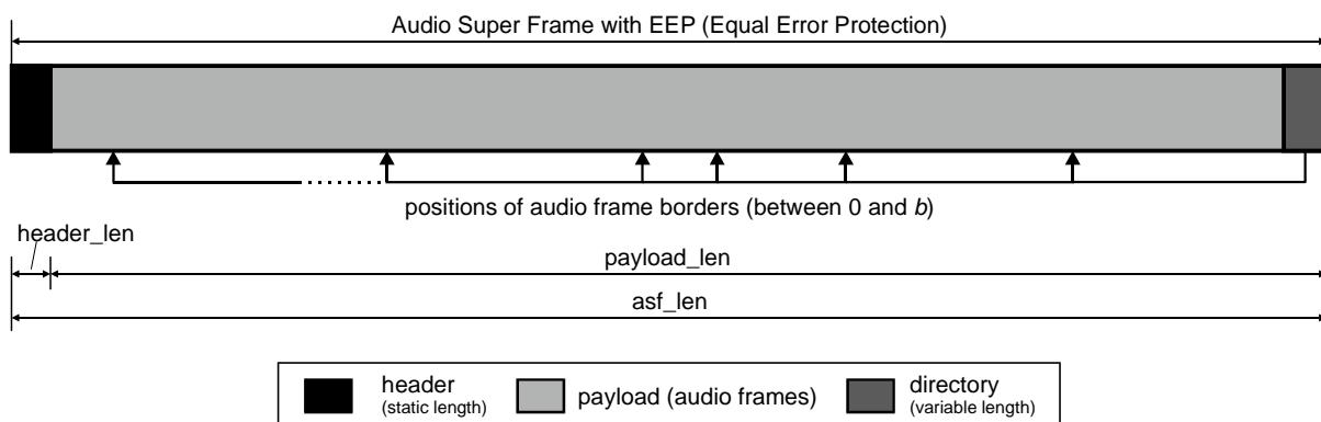
**Figure 4: Example for xHE-AAC audio super frame structure**
