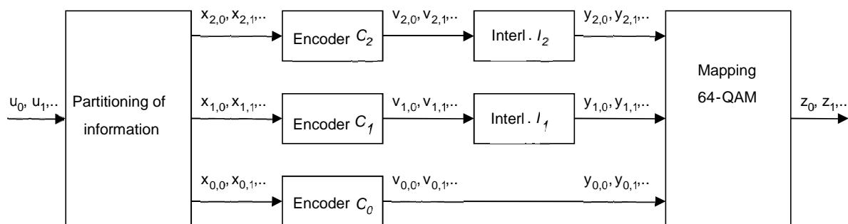
**Figure 20: Multilevel coding with 3 levels**
