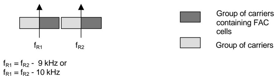
**Figure K.6: Example of base/enhancement DRM signals**
