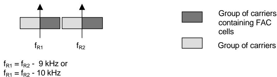
Figure K.6: Example of base/enhancement DRM signals
