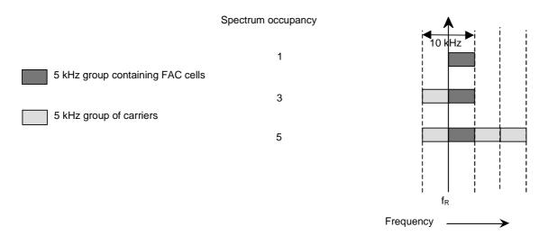
Figure 38: Spectrum occupancy for 10 kHz channels
