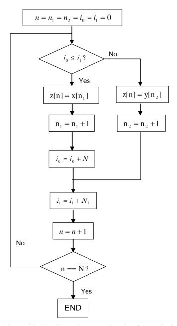
Figure 10: Flowchart of category interleaving method
