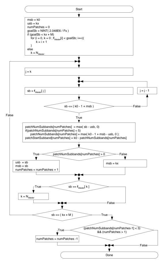
Figure 14: Flowchart of patch construction
