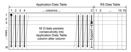
Figure 20: Placing data packets into FEC frame
