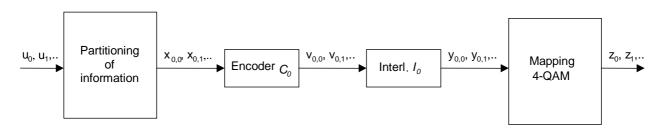
Figure 30: Multilevel coding with 1 level (SM)
