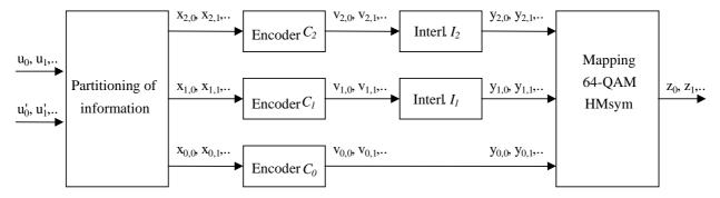
Figure 27: Multilevel coding with 3 levels for HMsym
