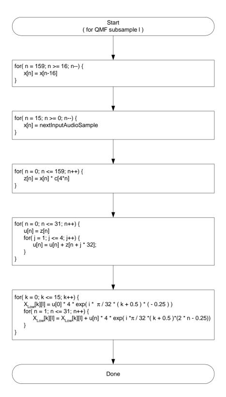
Figure 13: Flowchart of decoder 16-channel analysis QMF bank
