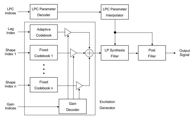
Figure 5: Block diagram of a CELP decoder
