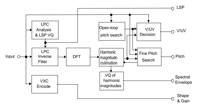
Figure 8: Block diagram of the HVXC encoder
