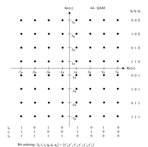
Figure 32: SM 64-QAM mapping with corresponding bit pattern
