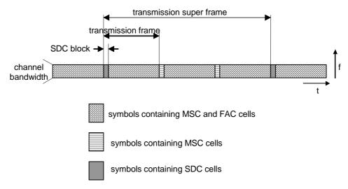
Figure 39: Time-frequency location of FAC and SDC signals
