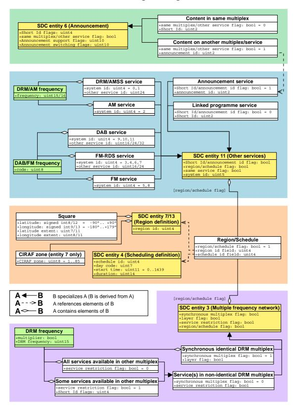
Figure F.1: Alternative Frequency and Announcement Signalling - Involved SDC data entities
