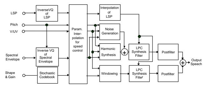
Figure 7: Block diagram of the HVXC decoder
