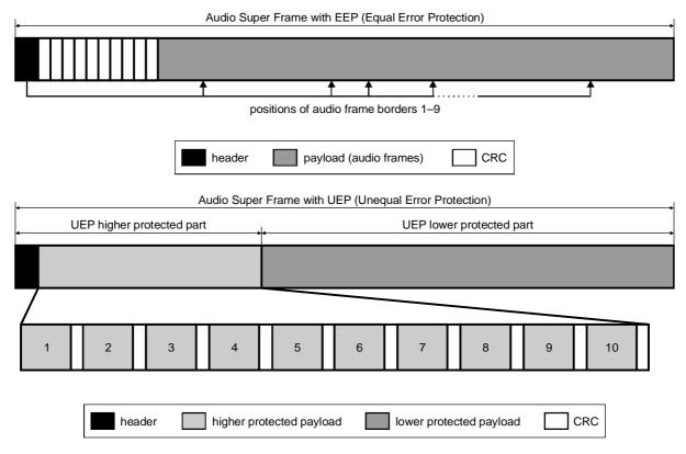
Figure 3: Example AAC audio super frame with 10 audio frames
