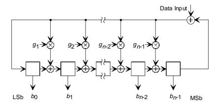
Figure D.1: General CRC block diagram
