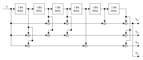
Figure 31: Convolutional encoder
