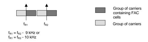
Figure K.6: Example of base/enhancement DRM signals
