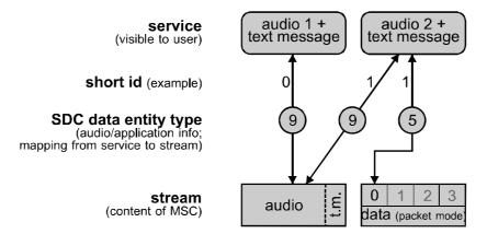
EXAMPLE 3: There is one audio service and one data service signalled to the user. The DRM multiplex consists of one audio stream and one data stream in packet mode containing one sub-stream. The data service points to the data application carried in the one sub-stream of the data stream. The audio service points to the audio stream and additionally also to the one sub-stream of the data stream.
