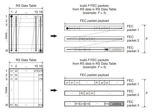
Figure 22: RS data byte order within FEC packets
