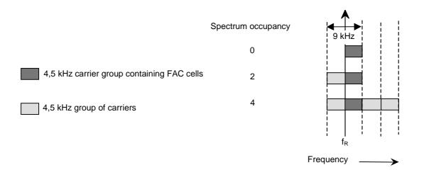
Figure 37: Spectrum occupancy for 9 kHz channels
