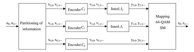
Figure 26: Multilevel coding with 3 levels for SM
