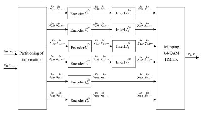
Figure 28: Multilevel coding with 3 levels for HMmix
