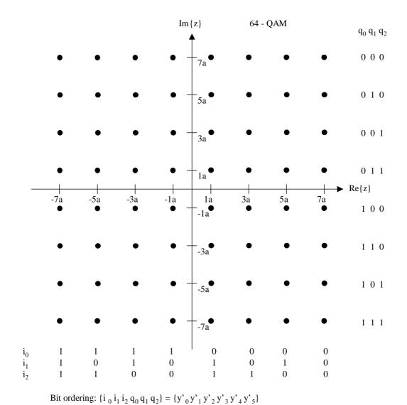
Figure 33: HMsym 64-QAM mapping with corresponding bit pattern
