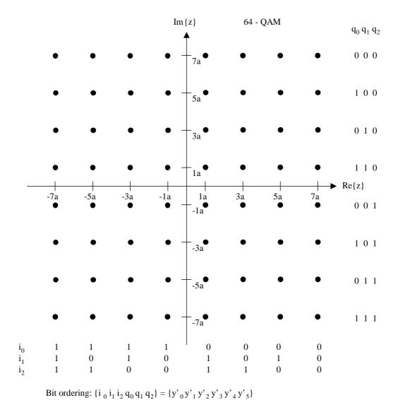
Figure 34: HMmix 64-QAM mapping with corresponding bit pattern
