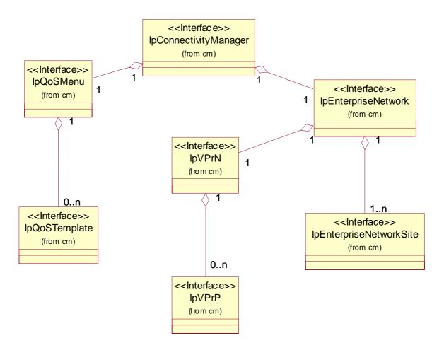
Figure 1: Connectivity Management High level class diagram
