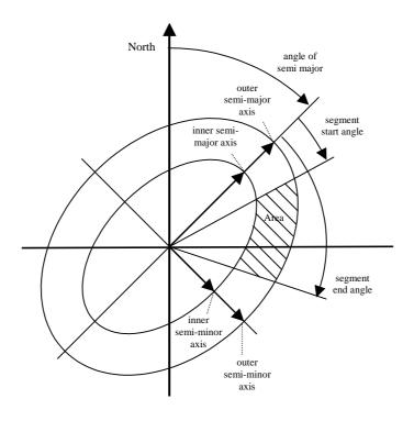
Figure 7: Description of an Ellipse Arc
