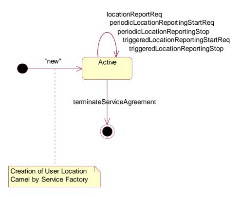
Figure 5: State Transition Diagram for User Location Camel
