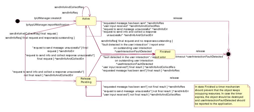
Figure 3: Application view on the UI object
