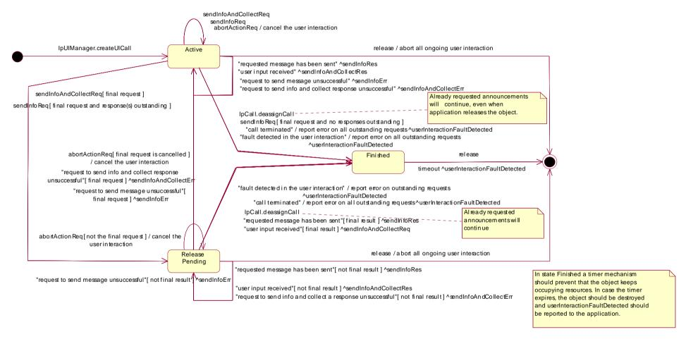
Figure 4: Application view on the UICall object
