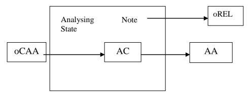
NOTE: The release event (oREL) can occur in any state resulting in a transition to Releasing state. Abbreviations used for the events:
