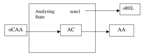
NOTE 1: The release event (oREL) can occur in any state resulting in a transition to Releasing state. Abbreviations used for the events:
