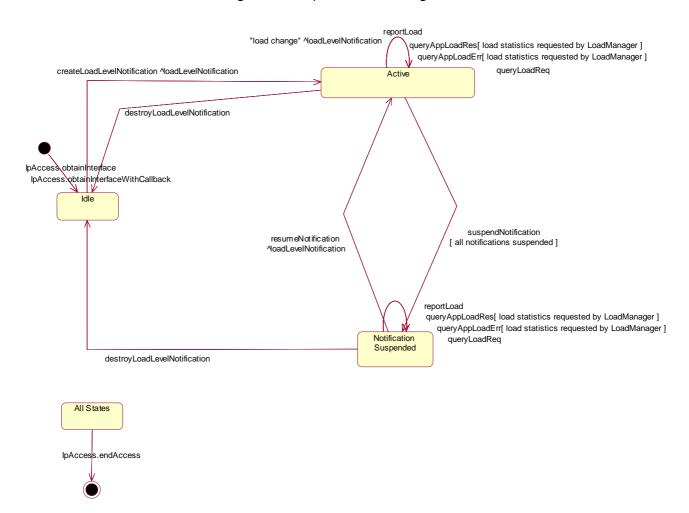
Figure 29: State Transition Diagram for IpFwLoadManager
