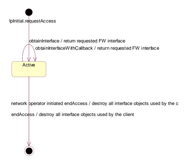
Figure 4: State Transition Diagram for IpAccess
