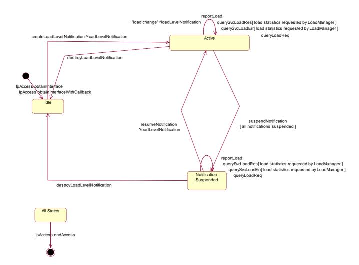
Figure 11: State Transition Diagram for IpLoadManager
