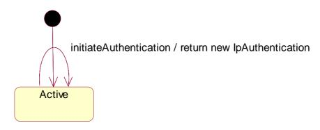
Figure 2: State Transition Diagram for IpInitial
