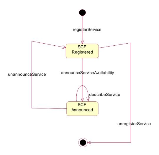
Figure 28: State Transition Diagram for IpFwServiceRegistration
