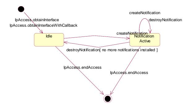
Figure 15: State Transition Diagram for IpEventNotification
