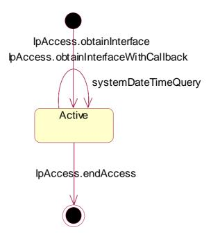
Figure 13: State Transition Diagram for IpOAM
