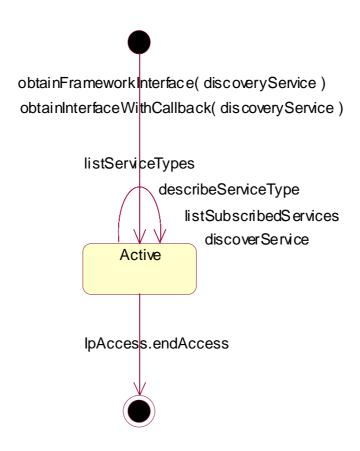
Figure 10: State Transition Diagram for IpServiceDiscovery
