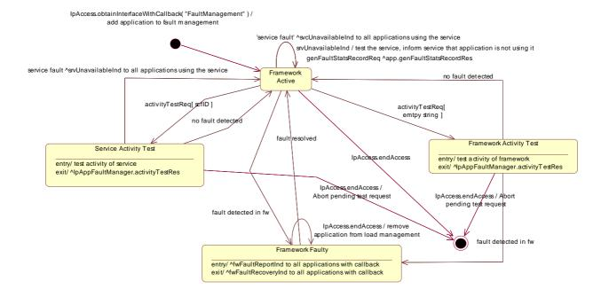
Figure 14: State Transition Diagram for IpFaultManager
