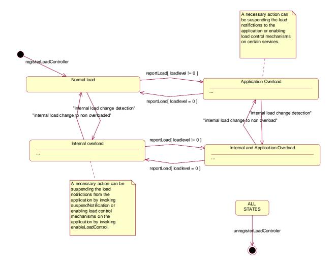
Figure 12: State Transition Diagram for LoadManagerInternal
