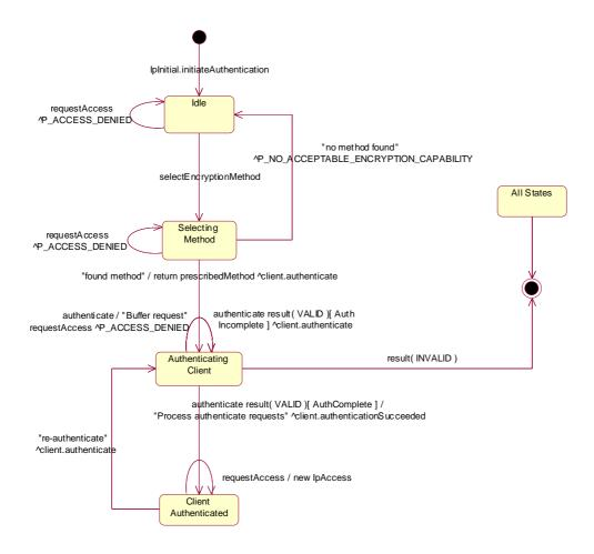
Figure 3: State Transition Diagram for IpAPILevelAuthentication
