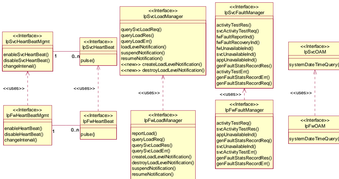
Figure 26: Integrity Management Package Overview
