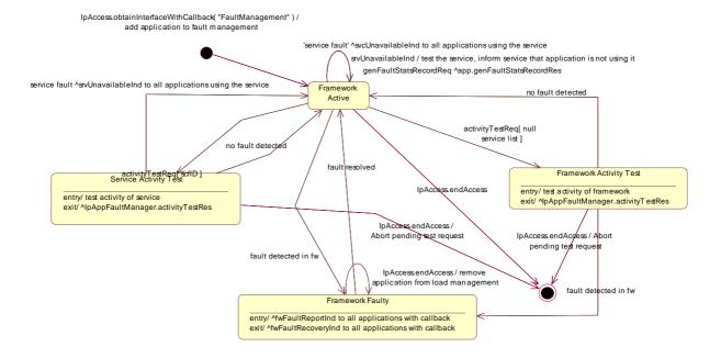
Figure 14: State Transition Diagram for IpFaultManager
