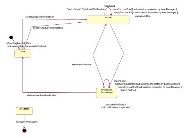
Figure 11: State Transition Diagram for IpLoadManager
