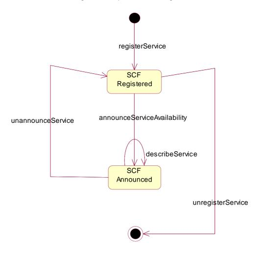
Figure 28: State Transition Diagram for IpFwServiceRegistration
