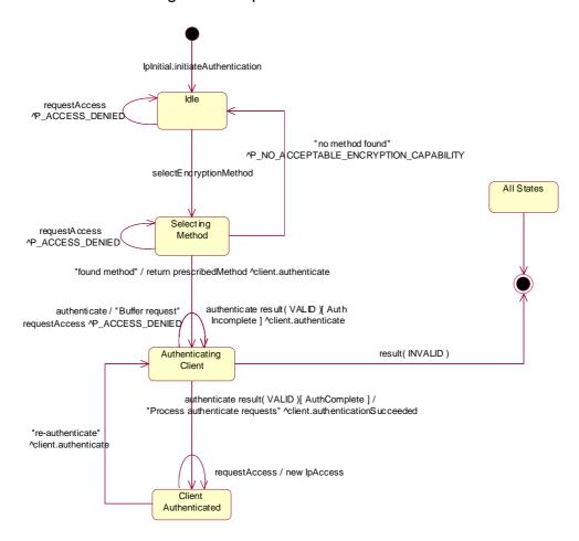
Figure 3: State Transition Diagram for IpAPILevelAuthentication
