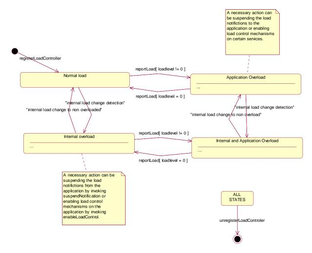
Figure 12: State Transition Diagram for LoadManagerInternal
