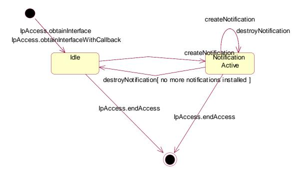
Figure 15: State Transition Diagram for IpEventNotification
