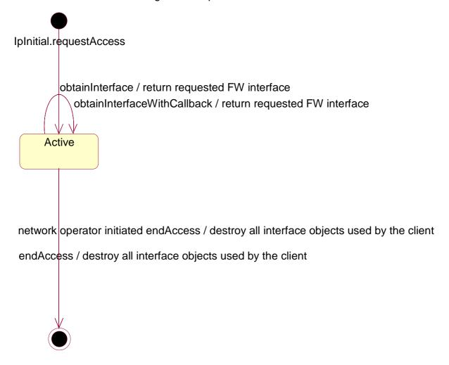
Figure 4: State Transition Diagram for IpAccess
