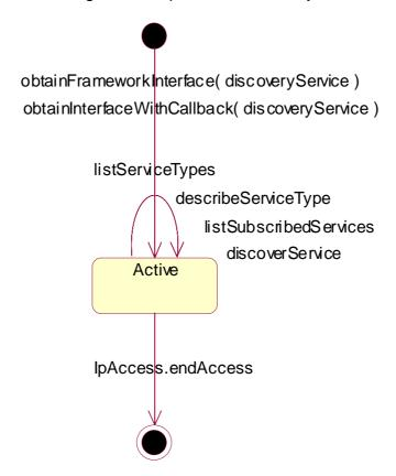
Figure 10: State Transition Diagram for IpServiceDiscovery
