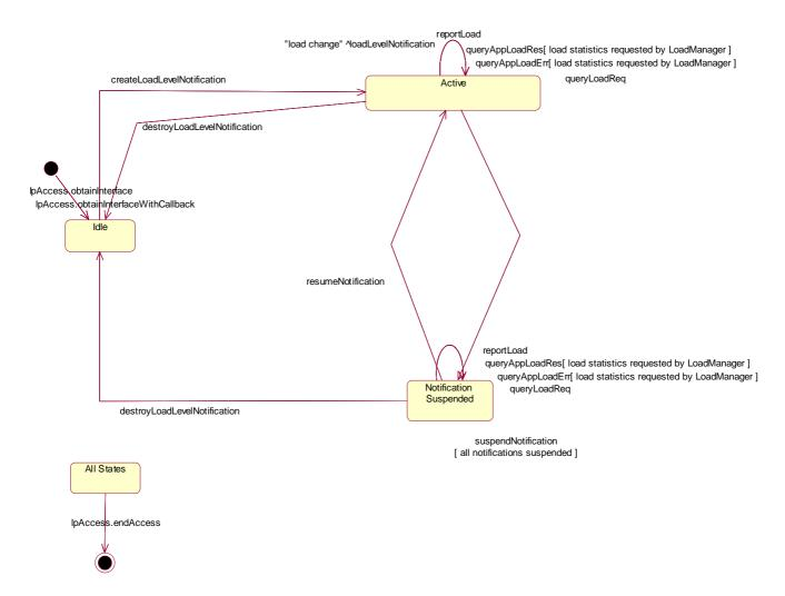
Figure 29: State Transition Diagram for IpFwLoadManager
