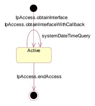
Figure 13: State Transition Diagram for IpOAM
