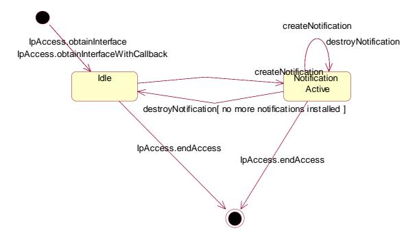
Figure 15: State Transition Diagram for IpEventNotification
