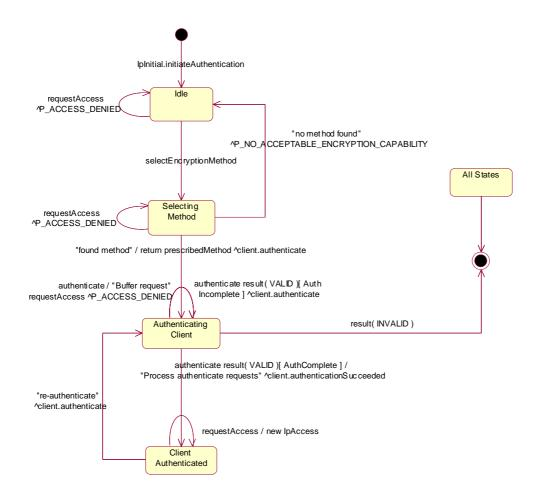
Figure 3: State Transition Diagram for IpAPILevelAuthentication
