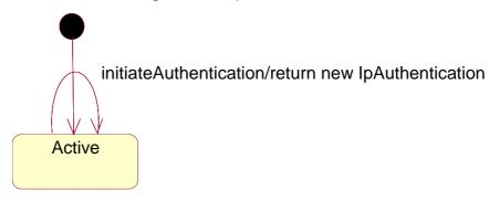
Figure 2: State Transition Diagram for IpInitial
