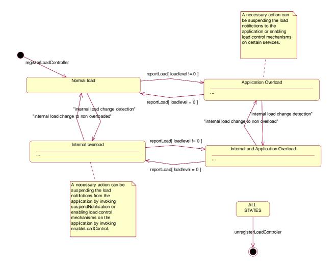
Figure 12: State Transition Diagram for LoadManagerInternal
