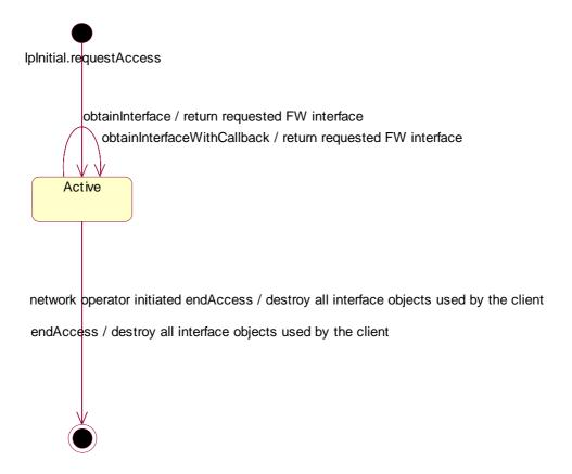
Figure 4: State Transition Diagram for IpAccess
