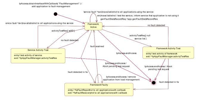
Figure 14: State Transition Diagram for IpFaultManager
