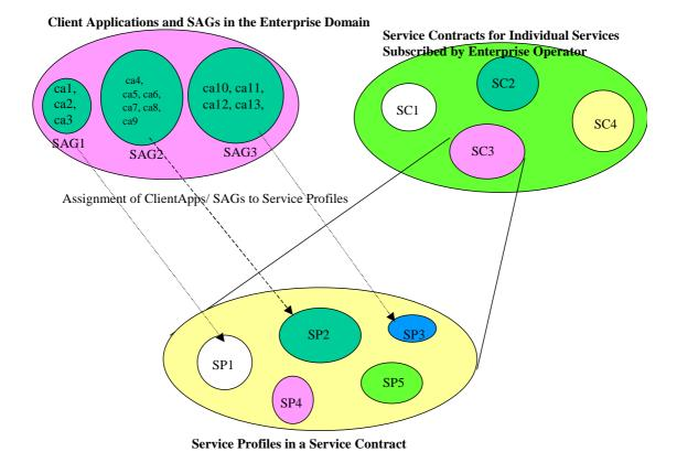
Figure 17: Relationship between Client Applications/SAG, Service Contract and Service Profiles
