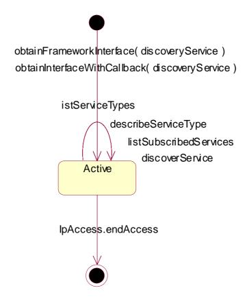
Figure 10: State Transition Diagram for IpServiceDiscovery
