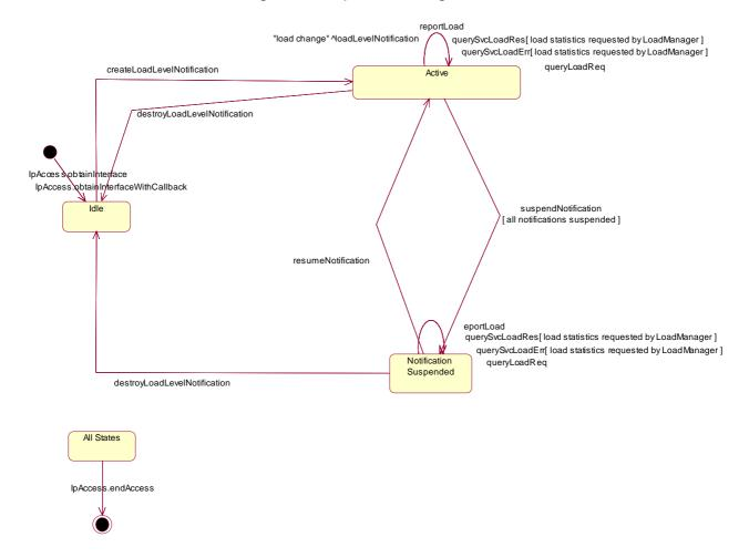
Figure 11: State Transition Diagram for IpLoadManager
