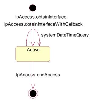
Figure 13: State Transition Diagram for IpOAM
