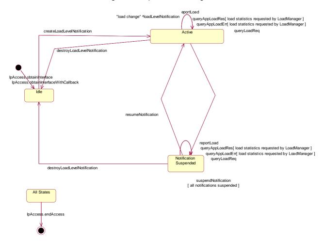
Figure 29: State Transition Diagram for IpFwLoadManager
