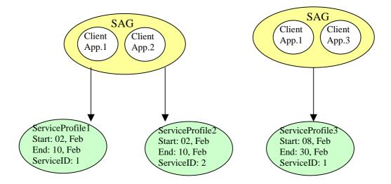
Figure 18: Overlapping date fields in service profiles
