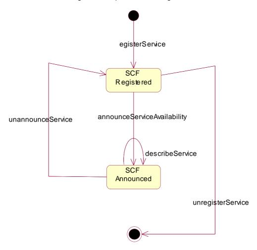
Figure 28: State Transition Diagram for IpFwServiceRegistration
