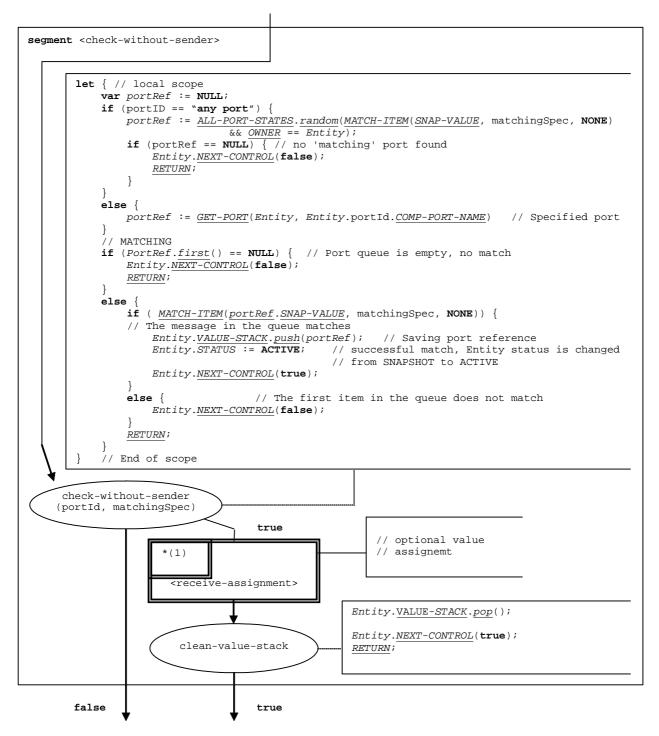
Figure 58: Flow graph segment <check-without-sender>
