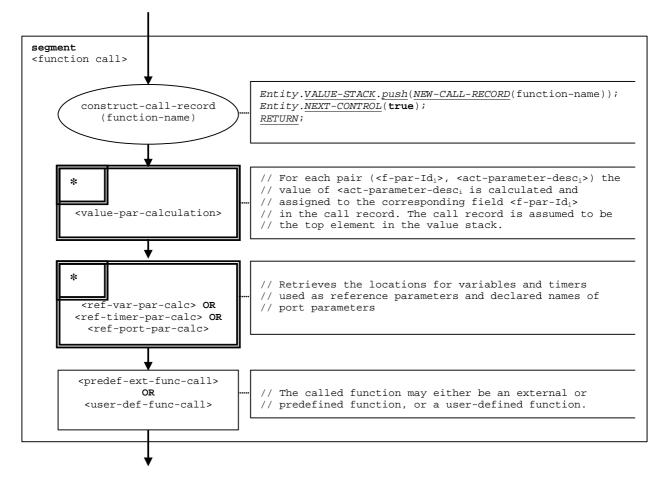
Figure 80: Flow graph segment <function-call>
