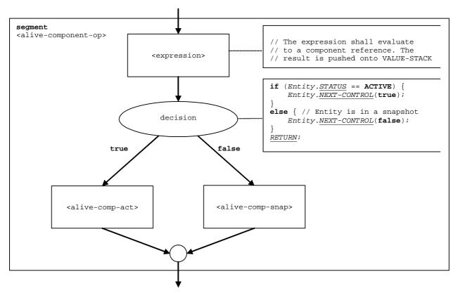
Figure 37a: Flow graph segment <alive-component-op>
