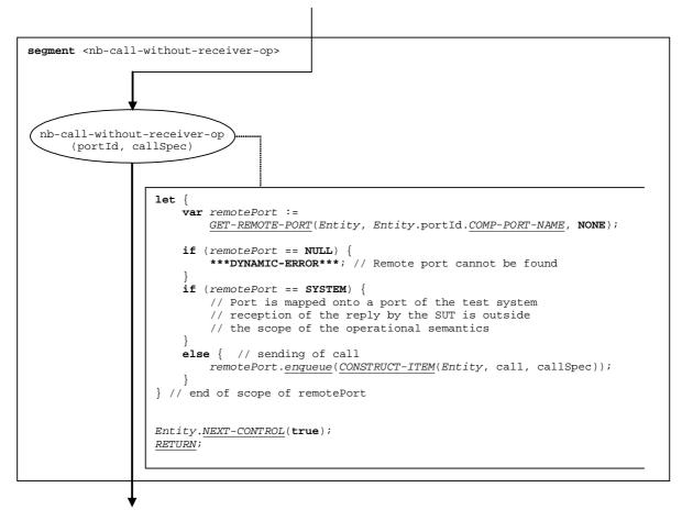
Figure 50: Flow graph segment <nb-call-without-receiver>
