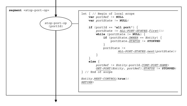
Figure 129: Flow graph segment <stop-port-op>
