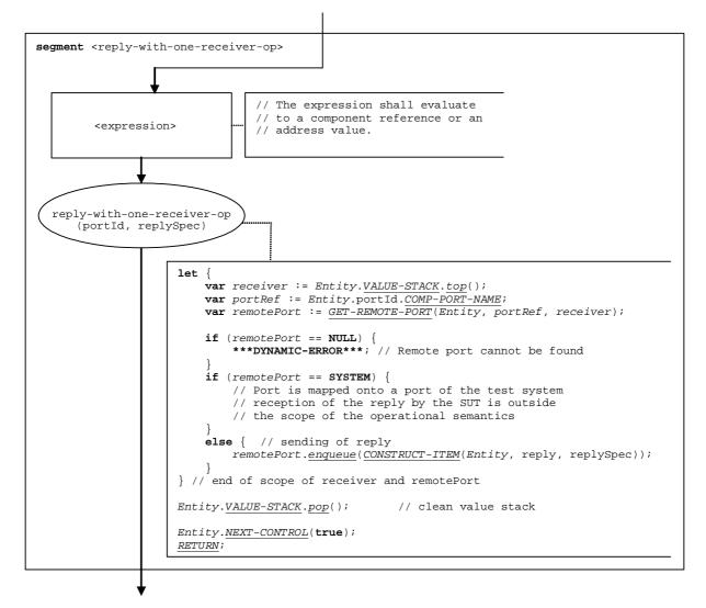
Figure 106: Flow graph segment <reply-with-one-receiver-op>
