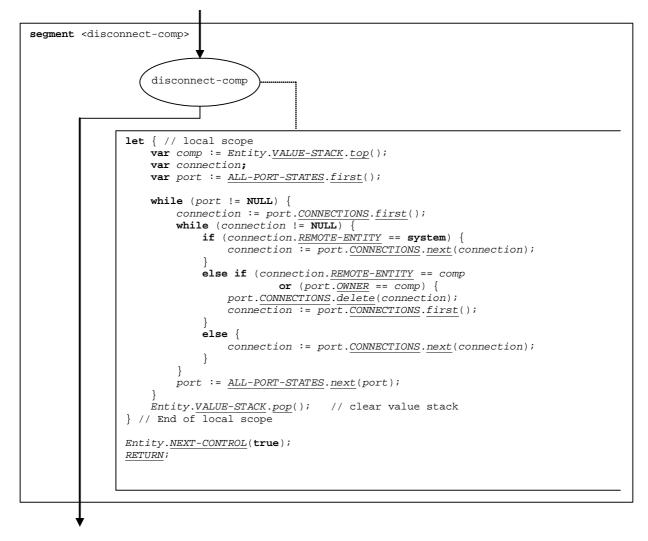
Figure 64c: Flow graph segment <disconnect-comp>
