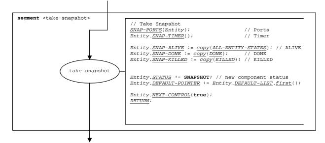
Figure 39: Flow graph segment <take-snapshot>
