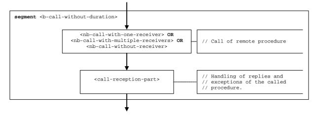
Figure 51: Flow graph segment <b-call-without-duration>
