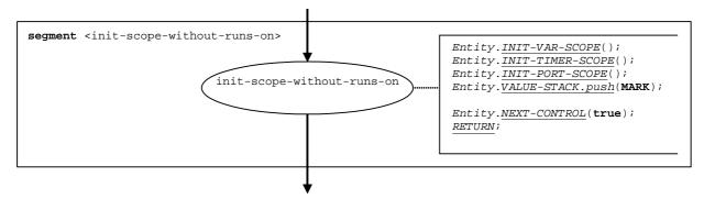
Figure 76b: Flow graph segment <init-scope-without-runs-on>
