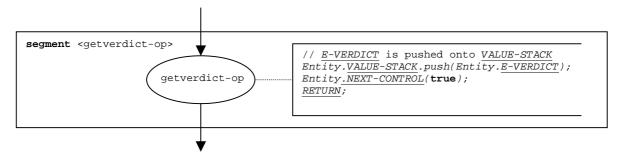
Figure 88: Flow graph segment <getverdict-op>
