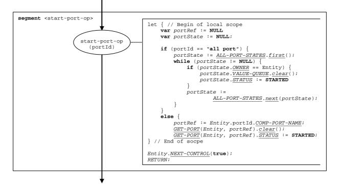
Figure 121: Flow graph segment <start-port-op>
