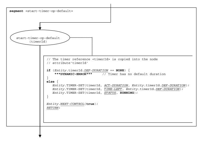
Figure 123: Flow graph segment <start-timer-op-default>
