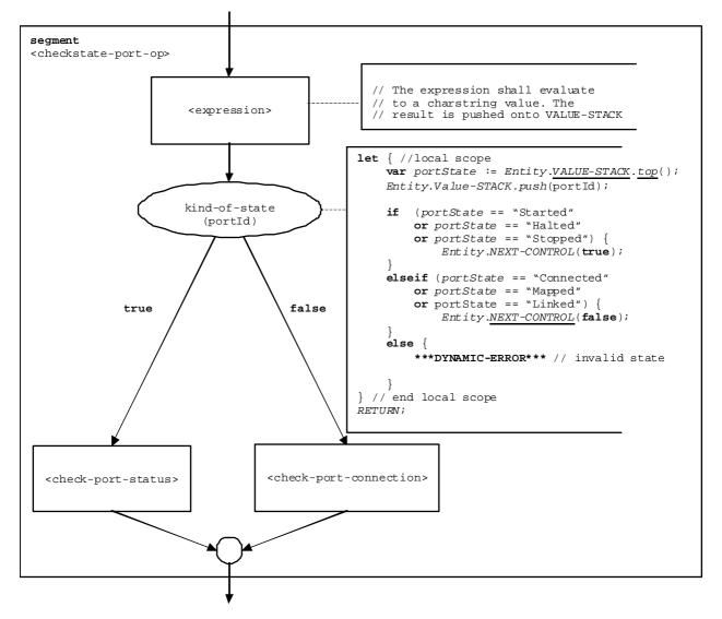
Figure 58a: Flow graph segment <checkstate-port-op>
