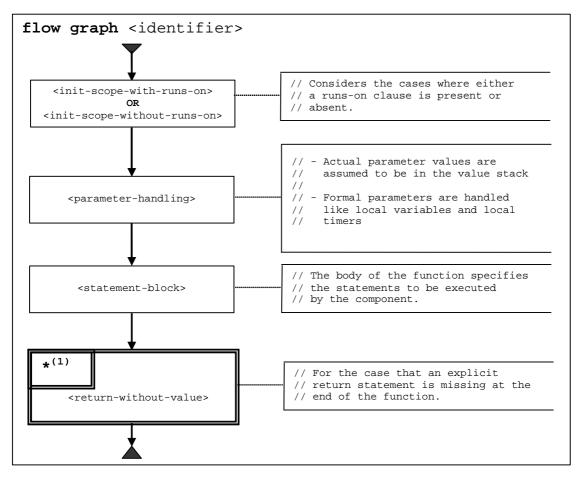
Figure 20: Flow graph representation of functions
