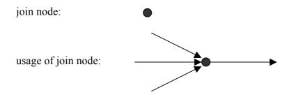
Figure 15b: Joining of flow lines
