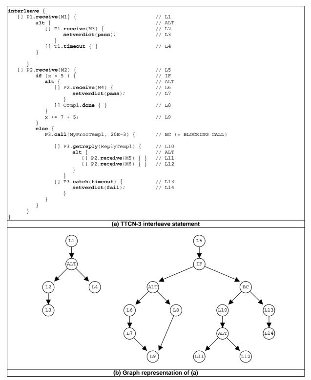
Figure 6: Graph representation of a TTCN-3 interleave statement
