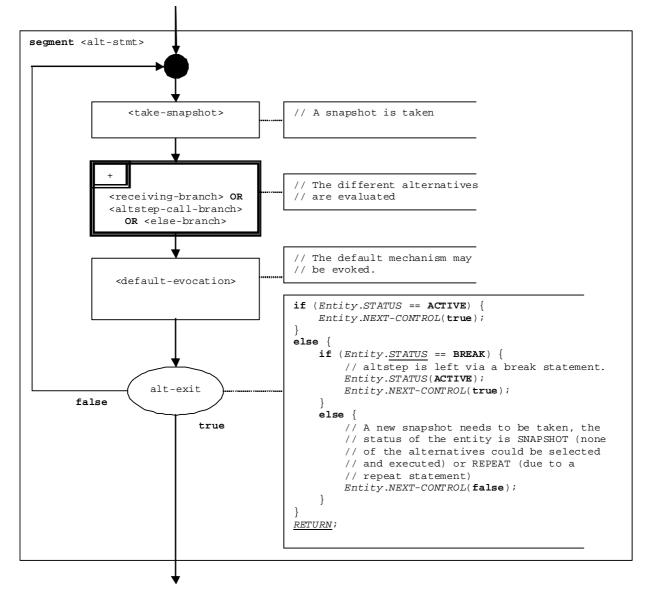
Figure 38: Flow graph segment <alt-stmt>
