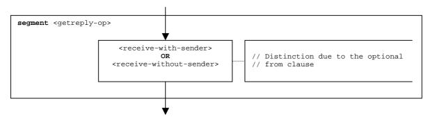
Figure 87: Flow graph segment <getreply-op>
