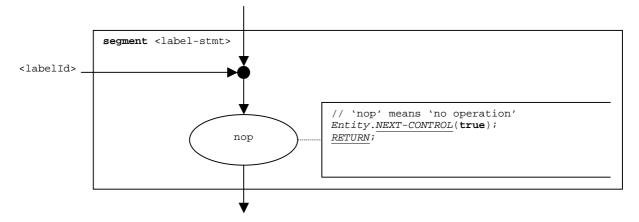
Figure 91: Flow graph segment <label-stmt>
