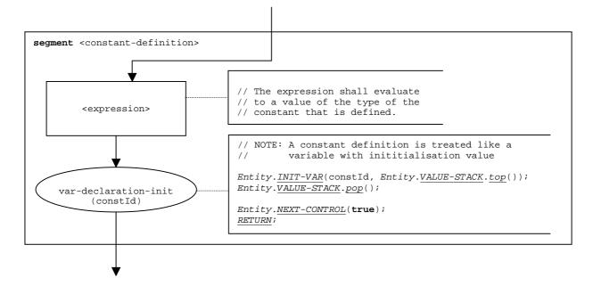
Figure 61: Flow graph segment <constant-definition>
