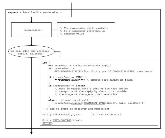
Figure 49: Flow graph segment <nb-call-with-one-receiver>
