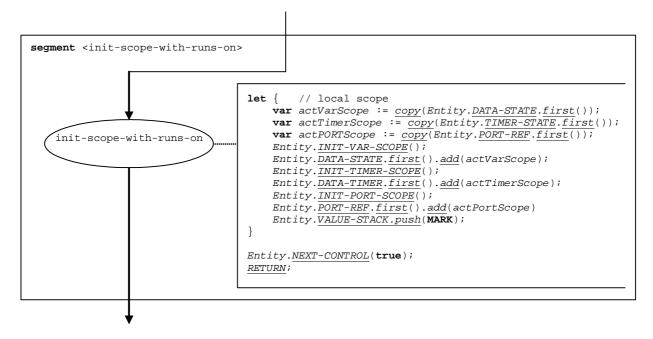
Figure 76a: Flow graph segment <init-scope-with-runs-on>
