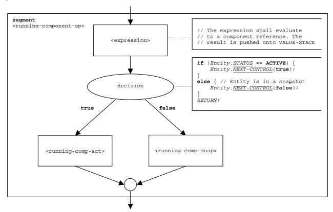
Figure 111: Flow graph segment <running-component-op>
