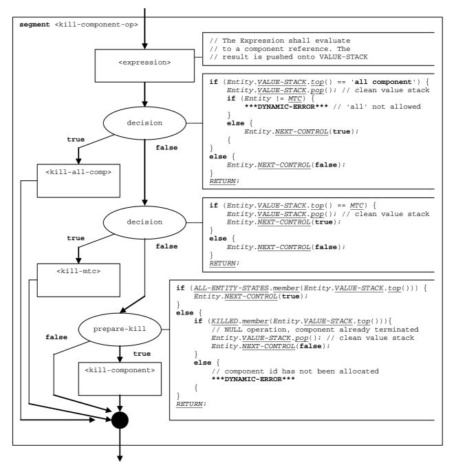
Figure 90a: Flow graph segment <kill-component-op>
