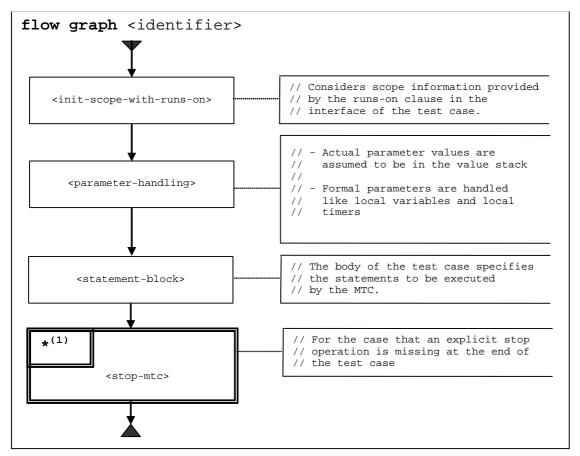
Figure 19: Flow graph representation of test cases
