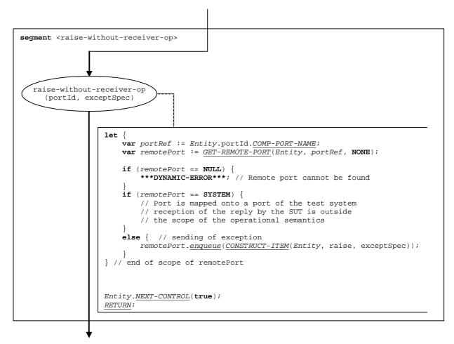
Figure 98: Flow graph segment <raise-without-receiver-op>
