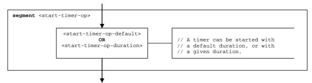
Figure 122: Flow graph segment <start-timer-op>
