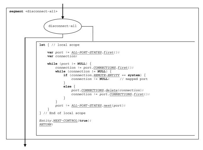
Figure 64b: Flow graph segment <disconnect-all>
