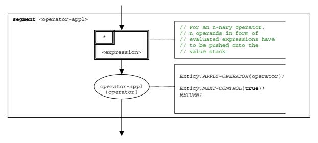
Figure 74: Flow graph segment <operator-appl>
