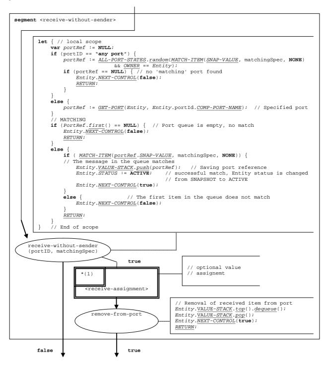
Figure 102: Flow graph segment <receive-without-sender>
