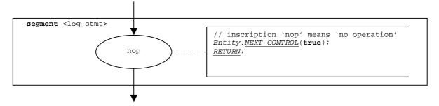
Figure 92: Flow graph segment <log-stmt>
