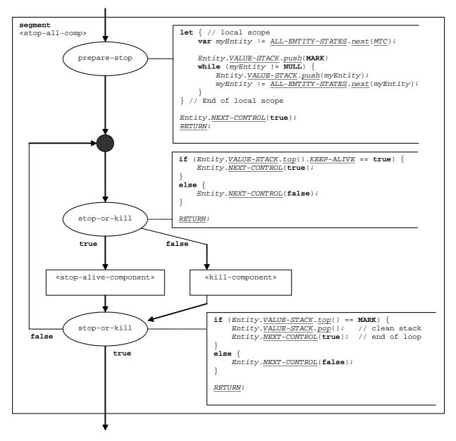
Figure 127: Flow graph segment <stop-all-comp>
