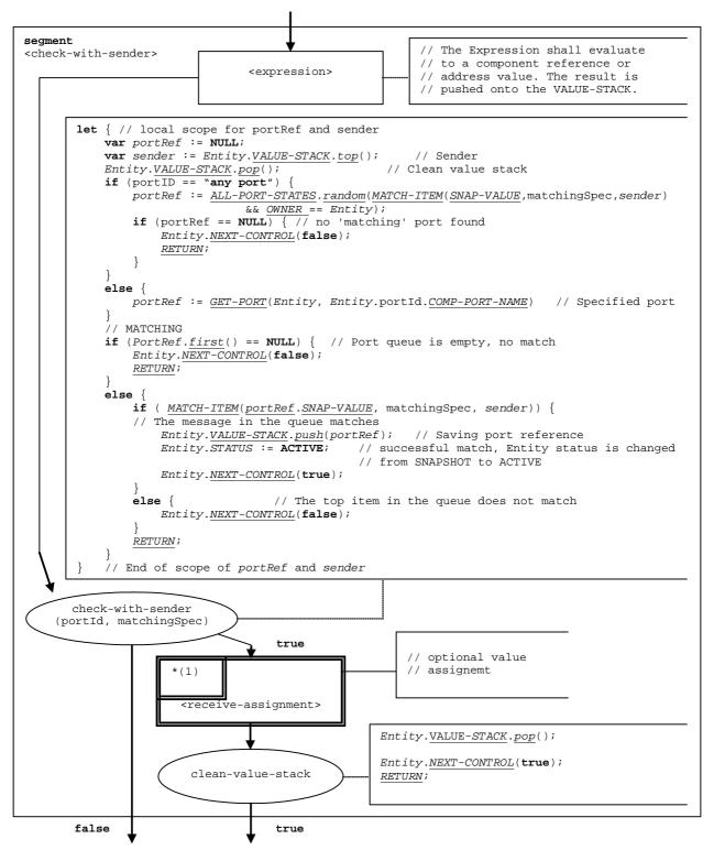
Figure 57: Flow graph segment <check-with-sender>
