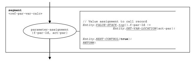
Figure 82: Flow graph segment <ref-par-var-calc>
