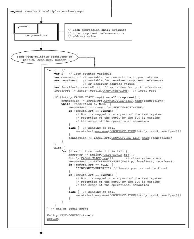
Figure 117a: Flow graph segment <send-with-multiple-receivers-op>
