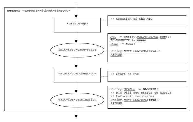
Figure 68: Flow graph segment <execute-without-timeout>
