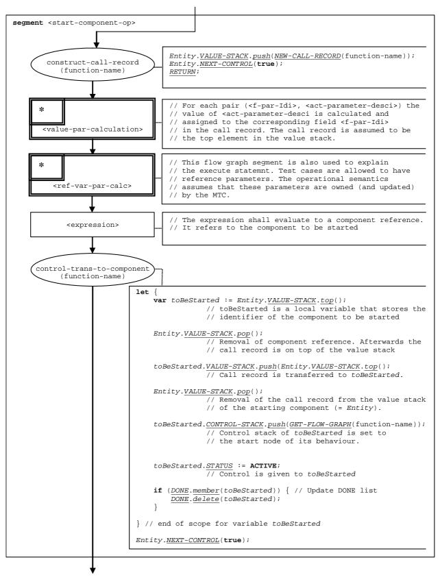
Figure 120: Flow graph segment <start-component-op>
