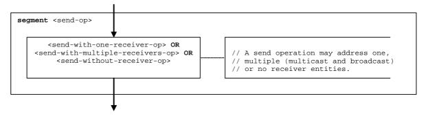
Figure 116: Flow graph segment <send-op>
