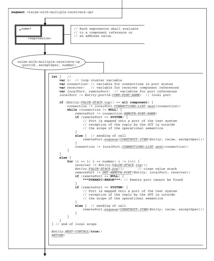
Figure 97a: Flow graph segment <raise-with-multiple-receivers-op>
