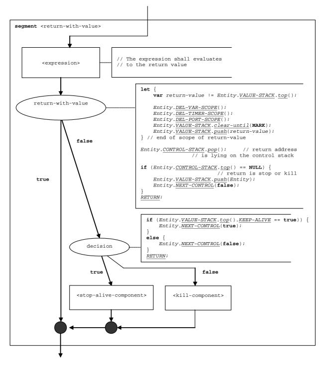
Figure 109: Flow graph segment <return-with-value>
