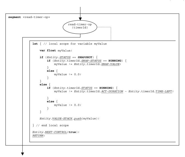
Figure 99: Flow graph segment <read-timer-op>
