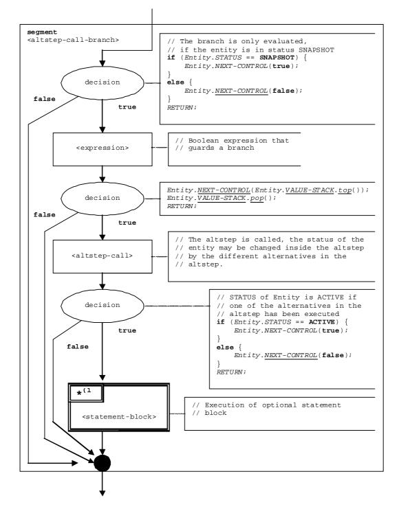
Figure 41: Flow graph segment <altstep-call-branch>
