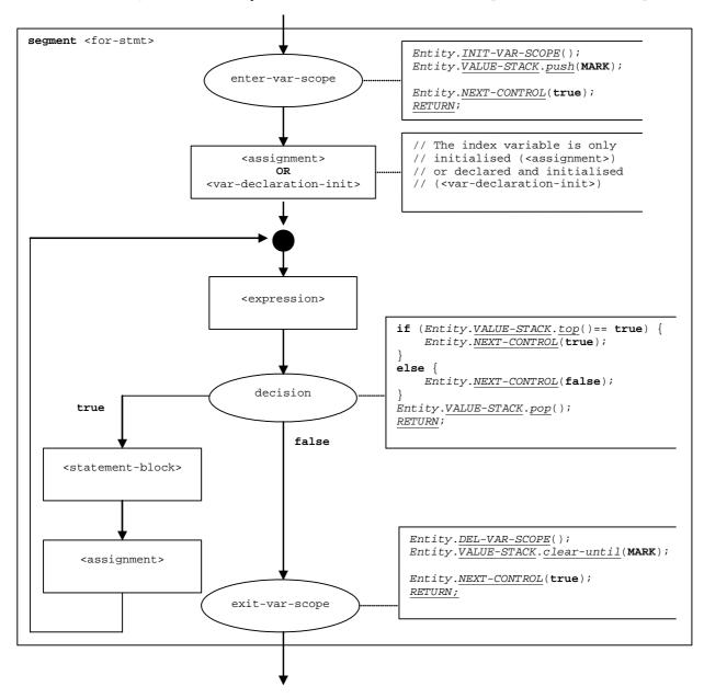
Figure 79: Flow graph segment <for-stmt>
