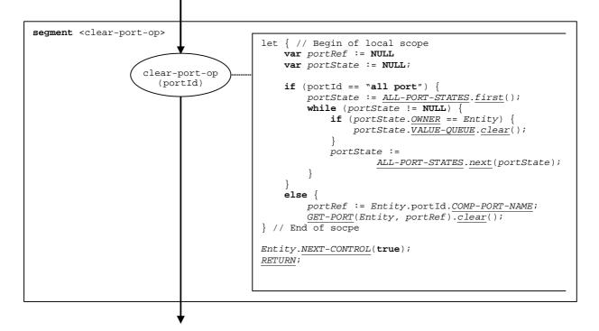
Figure 59: Flow graph segment <clear-port-op>
