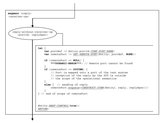
Figure 107: Flow graph segment <reply-without-receiver-op>
