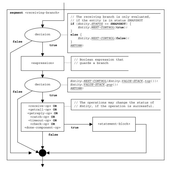
Figure 40: Flow graph segment <receiving-branch>
