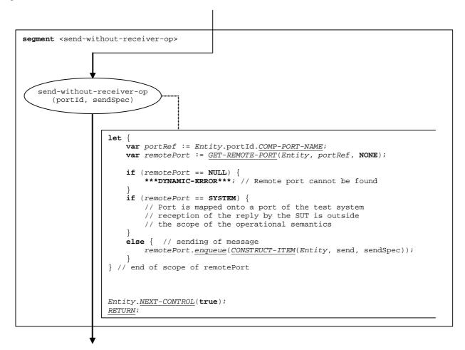
Figure 118: Flow graph segment <send-without-receiver-op>
