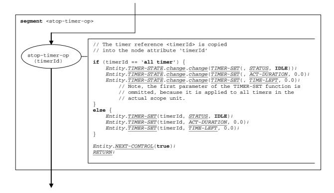
Figure 130: Flow graph segment <stop-timer-op>
