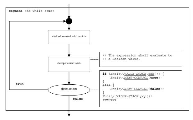
Figure 65: Flow graph segment <do-while-stmt>
