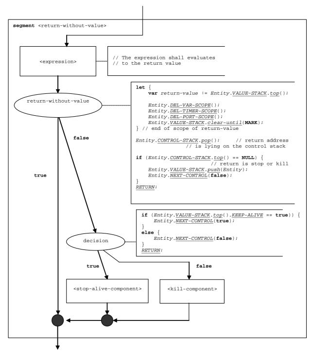
Figure 110: Flow graph segment <return-without-value>
