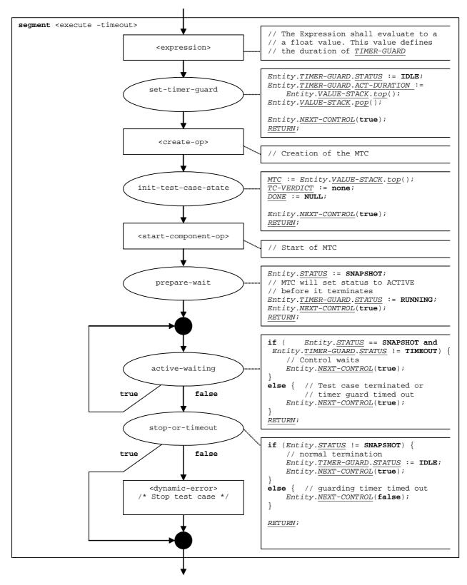
Figure 69: Flow graph segment <execute-timeout>
