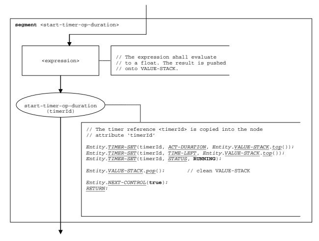
Figure 124: Flow graph segment <start-timer-op-duration>
