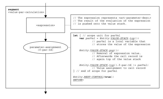
Figure 81: Flow graph segment <value-par-calculation>
