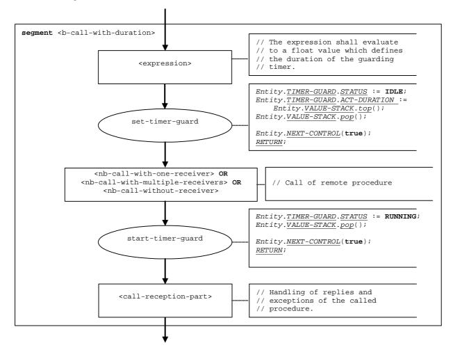
Figure 52: Flow graph segment <b-call-with-duration>
