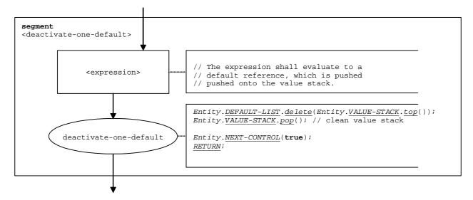
Figure 63b: Flow graph segment <deactivate-one-default>
