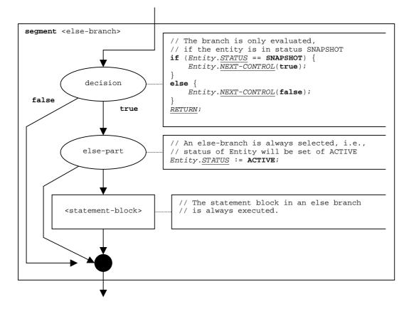
Figure 42: Flow graph segment <else-branch>
