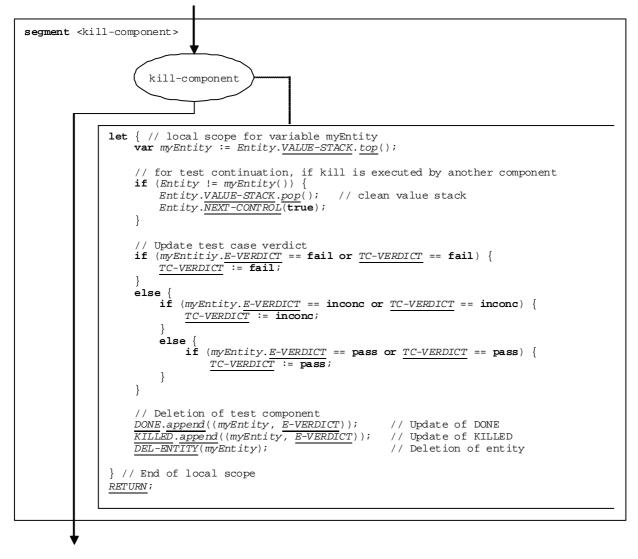
Figure 90c: Flow graph segment <kill-component>
