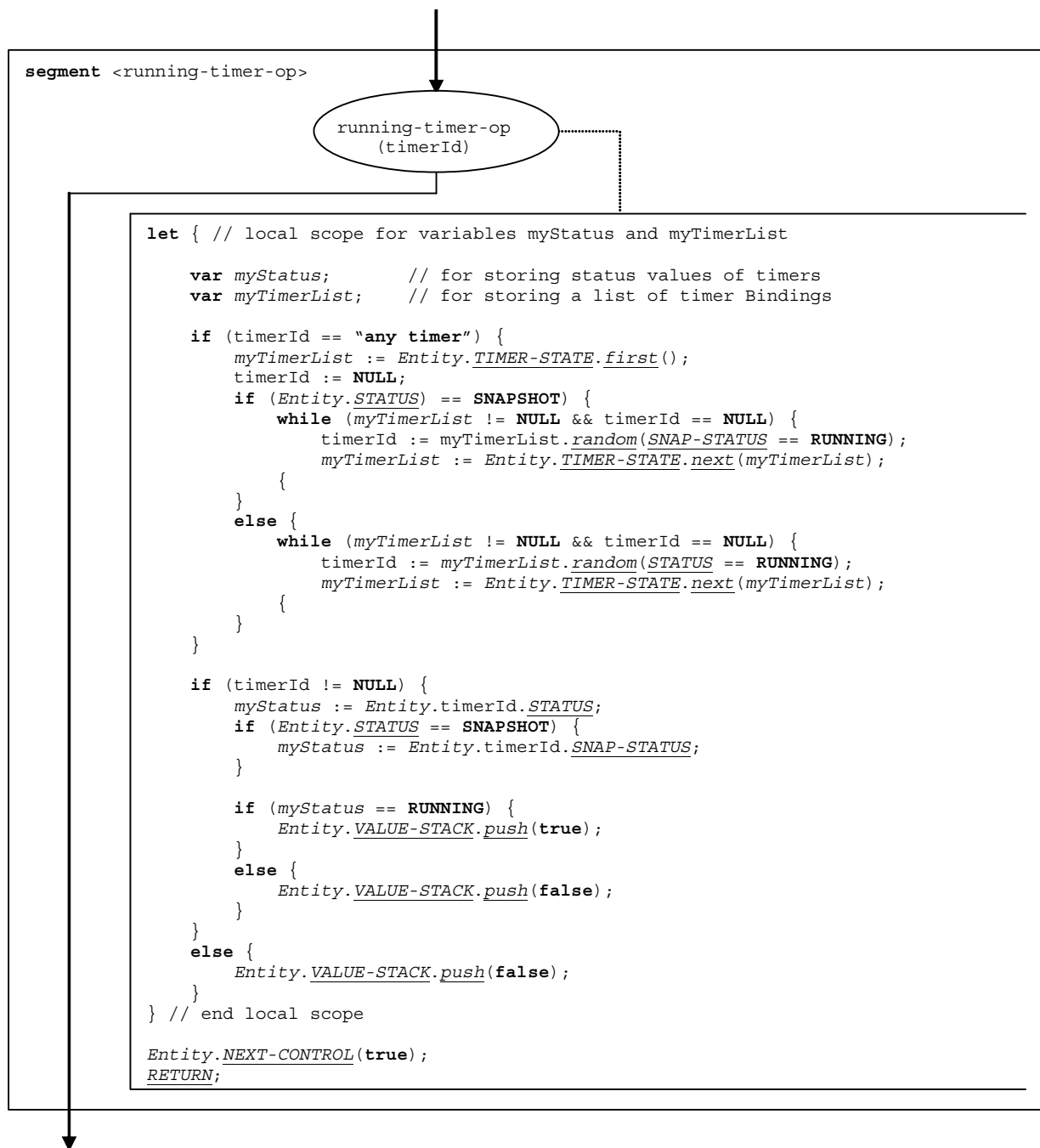
Figure 114: Flow graph segment <running-timer-op>
