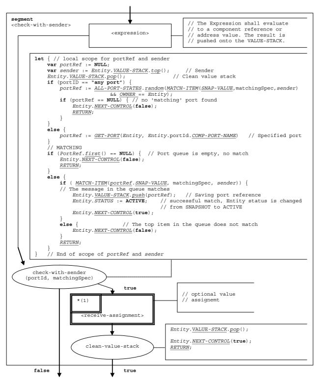
Figure 57: Flow graph segment <check-with-sender>
