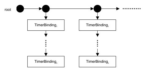
Figure 27: Structure of the TIMER-STATE part of an entity state
