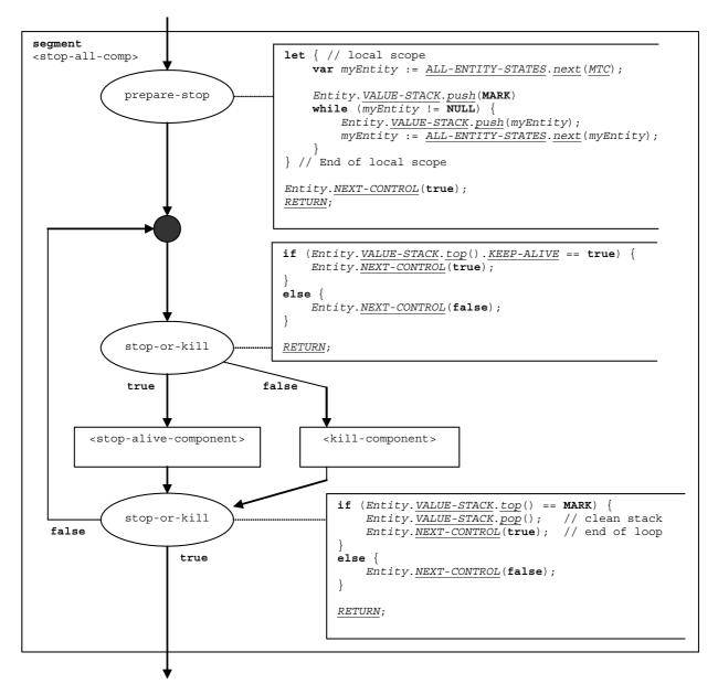
Figure 127: Flow graph segment <stop-all-comp>
