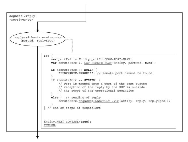
Figure 107: Flow graph segment <reply-without-receiver-op>
