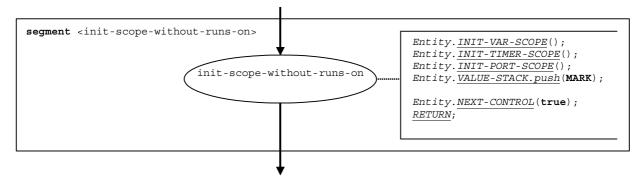
Figure 76b: Flow graph segment <init-scope-without-runs-on>
