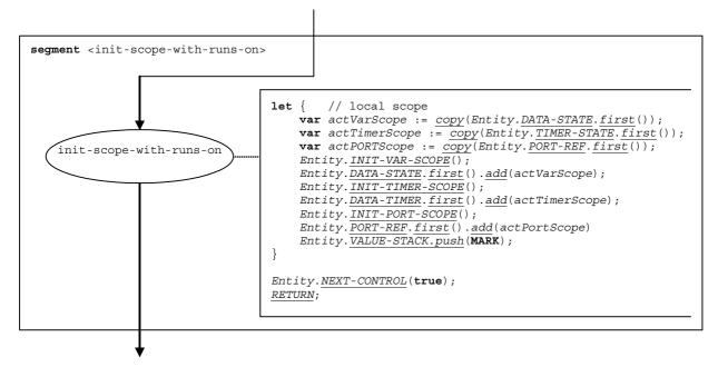
Figure 76a: Flow graph segment <init-scope-with-runs-on>
