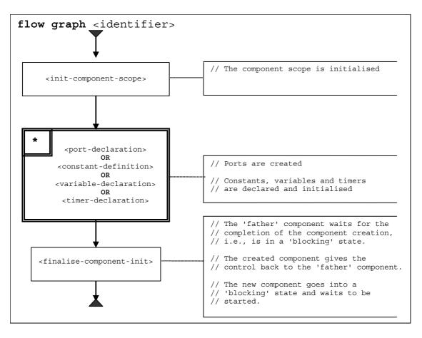
Figure 22: Flow graph representation of component type definitions
