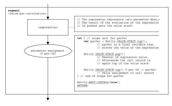
Figure 81: Flow graph segment <value-par-calculation>
