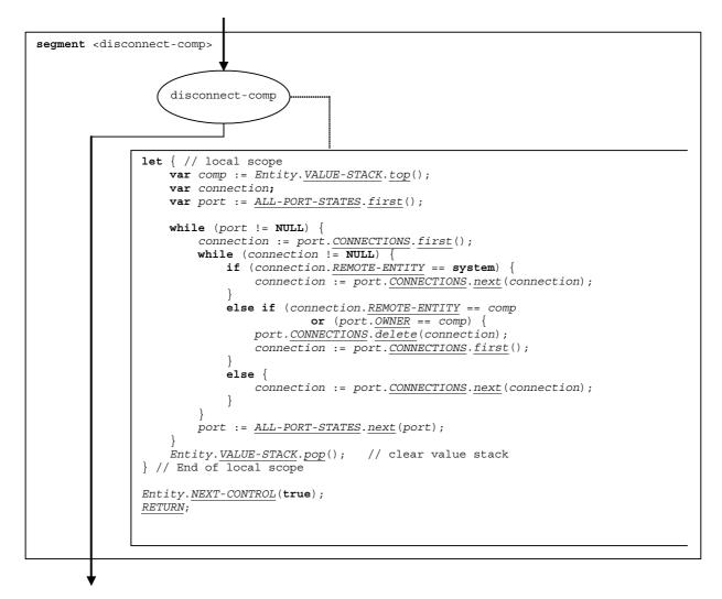
Figure 64c: Flow graph segment <disconnect-comp>
