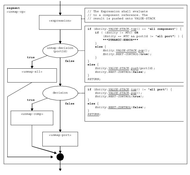
The execution of the **unmap** operation is defined by the flow graph segment <unmap-op> shown in figure 136.
