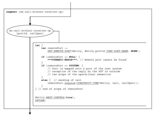
Figure 50: Flow graph segment <nb-call-without-receiver>
