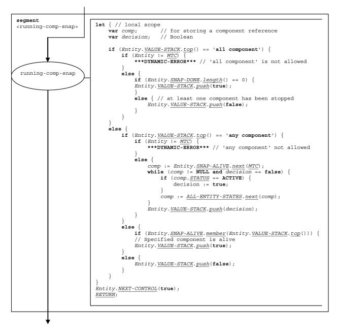
Figure 113: Flow graph segment <running-comp-snap>
