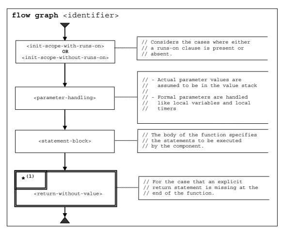
Figure 20: Flow graph representation of functions
