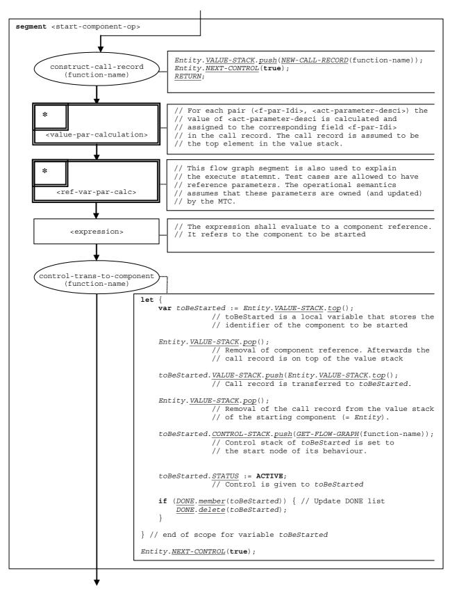
Figure 120: Flow graph segment <start-component-op>
