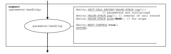
Figure 77: Flow graph segment <parameter-handling>
