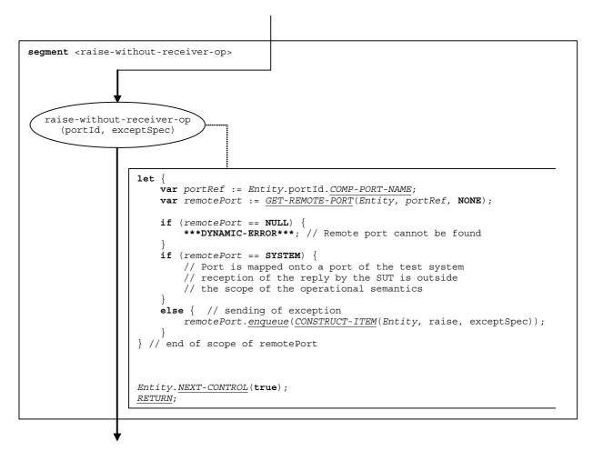
Figure 98: Flow graph segment <raise-without-receiver-op>
