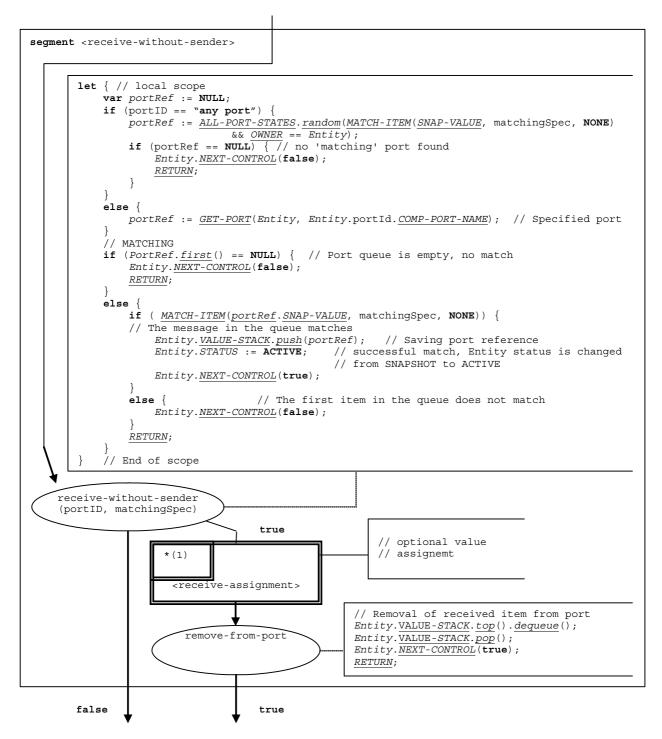
Figure 102: Flow graph segment <receive-without-sender>
