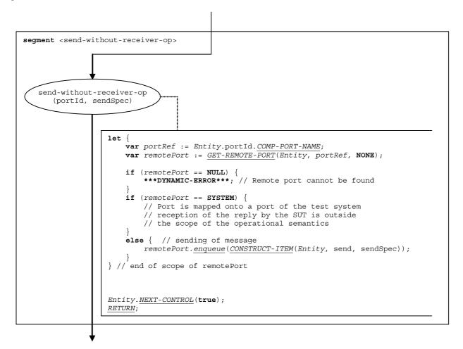
Figure 118: Flow graph segment <send-without-receiver-op>
