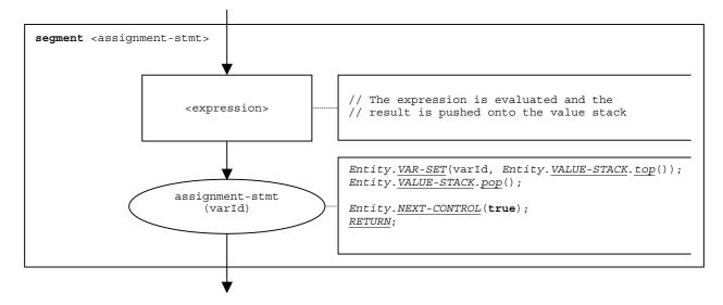
Figure 45: Flow graph segment <assignment-stmt>
