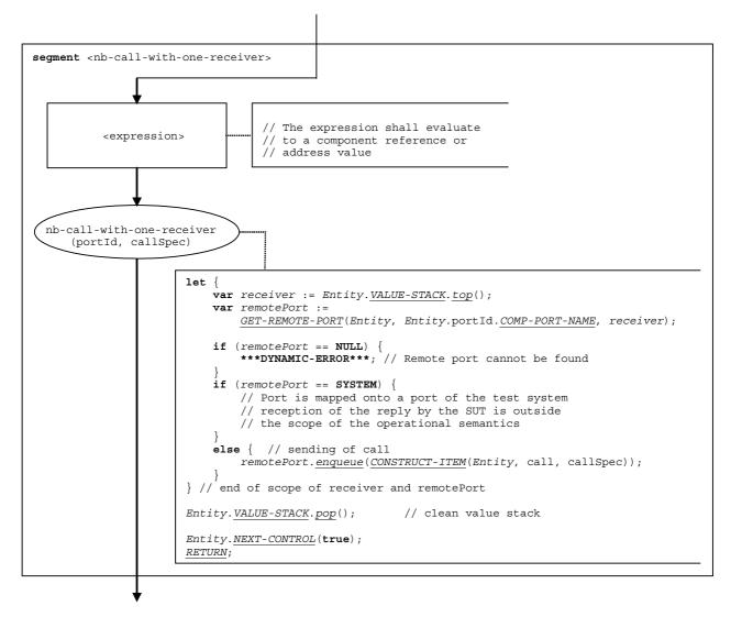
Figure 49: Flow graph segment <nb-call-with-one-receiver>
