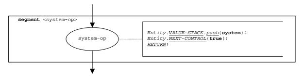
Figure 131: Flow graph segment <system-op>
