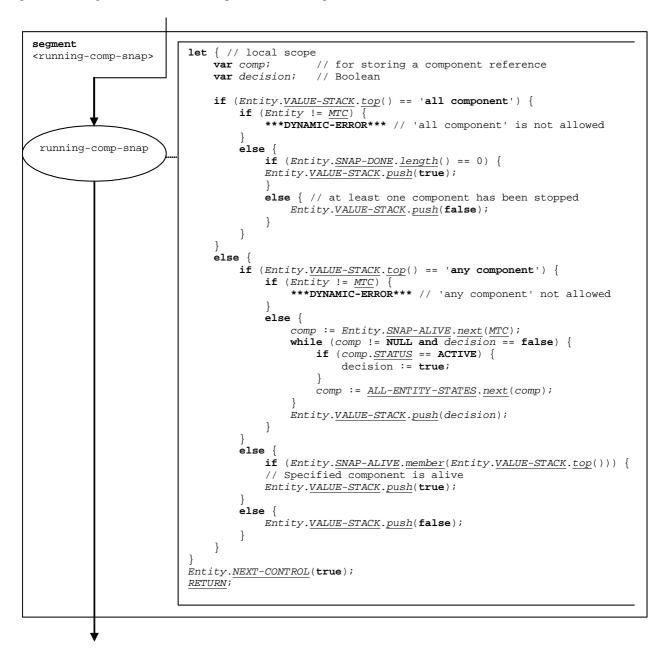
Figure 113: Flow graph segment <running-comp-snap>
