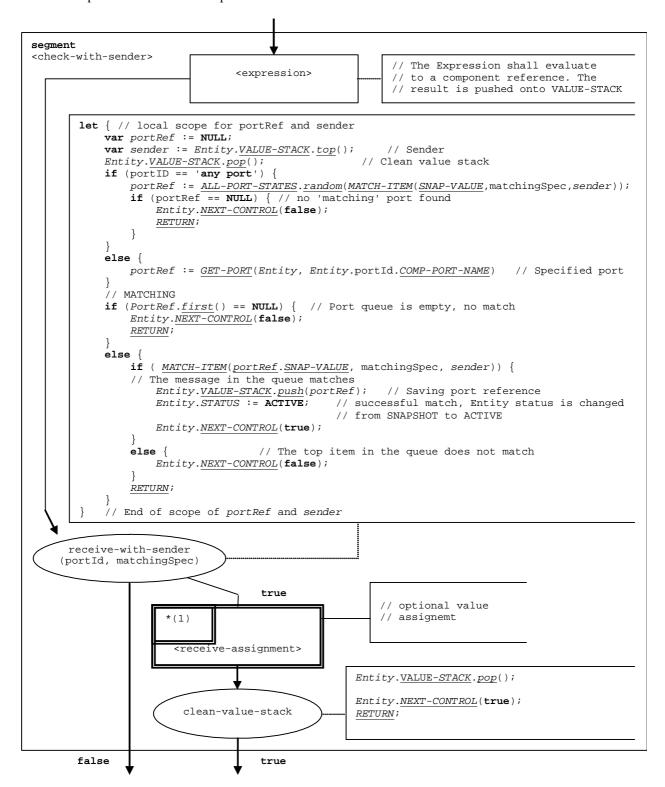
Figure 57: Flow graph segment <check-with-sender>
