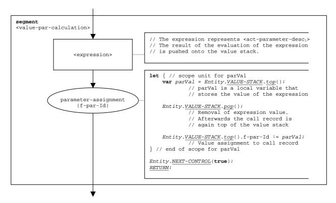
Figure 81: Flow graph segment <value-par-calculation>
