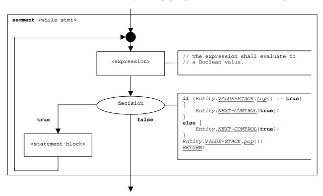
Figure 140: Flow graph segment <while-stmt>
