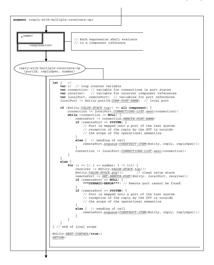
Figure 106a: Flow graph segment <reply-with-multiple-receivers-op>
