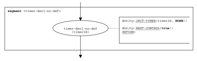
Figure 134: Flow graph segment <timer-decl-no-def>
