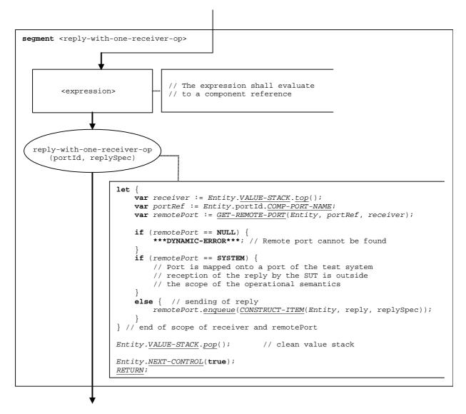
Figure 106: Flow graph segment <reply-with-one-receiver-op>
