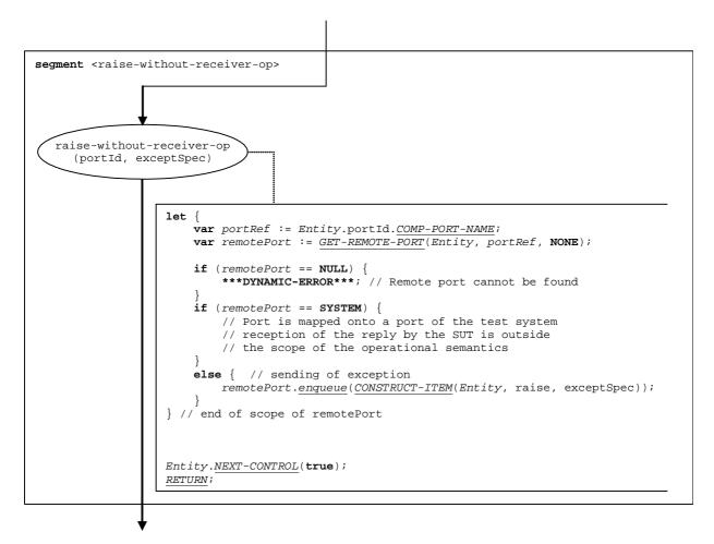
Figure 98: Flow graph segment <raise-without-receiver-op>
