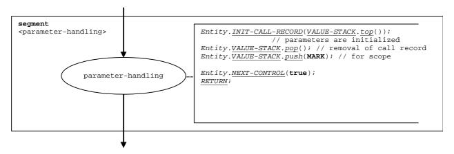
Figure 77: Flow graph segment cparameter-handling>
