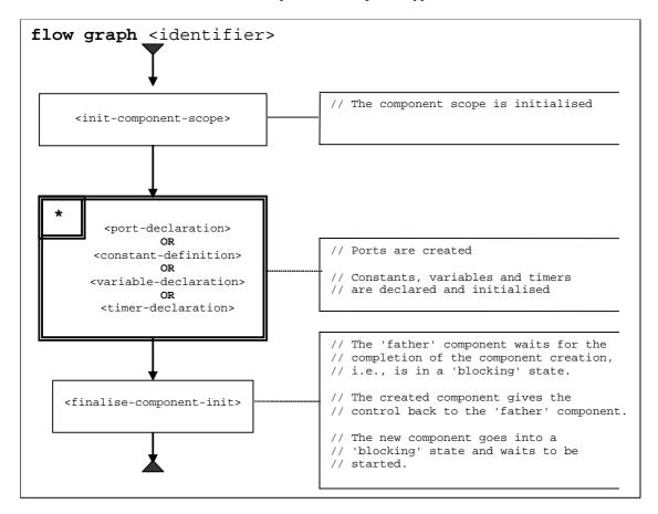
Figure 22: Flow graph representation of component type definitions
