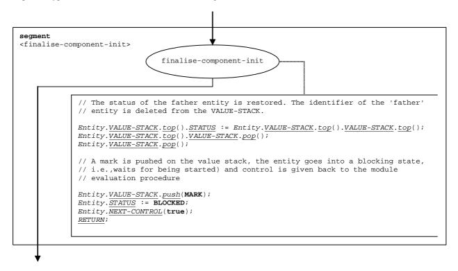
Figure 75: Flow graph segment <finalize-component-init>
