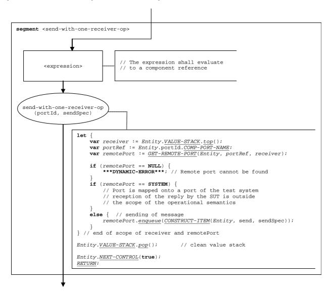
Figure 117: Flow graph segment <send-with-one-receiver-op>
