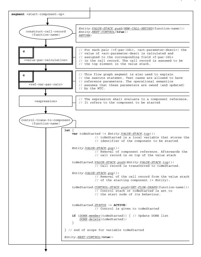
Figure 120: Flow graph segment <start-component-op>
