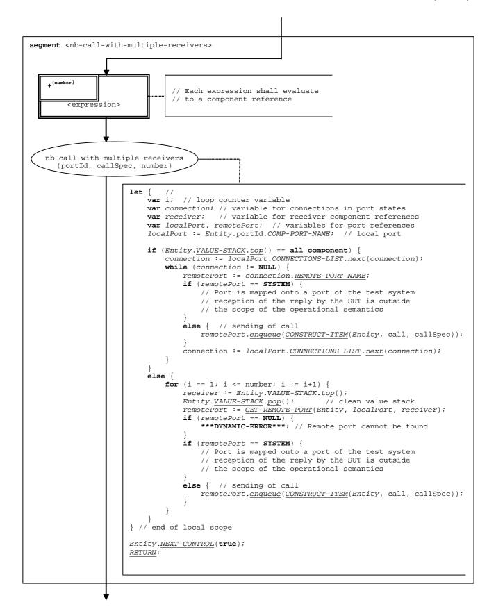
Figure 49a: Flow graph segment <nb-call-with-multiple-receivers>
