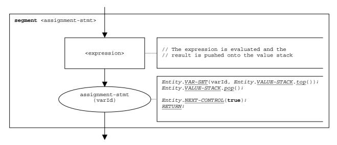
Figure 45: Flow graph segment <assignment-stmt>
