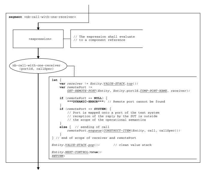
Figure 49: Flow graph segment <nb-call-with-receiver>
