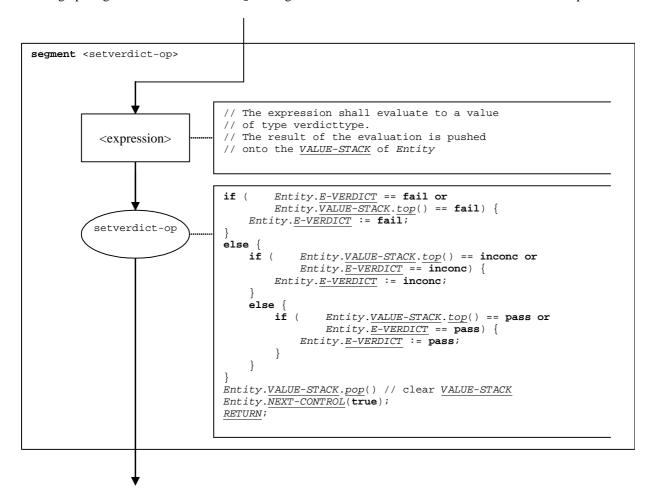
Figure 119: Flow graph segment <setverdict-op>
