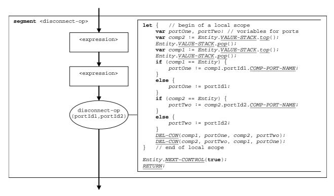
Figure 64: Flow graph segment < disconnect-op>
