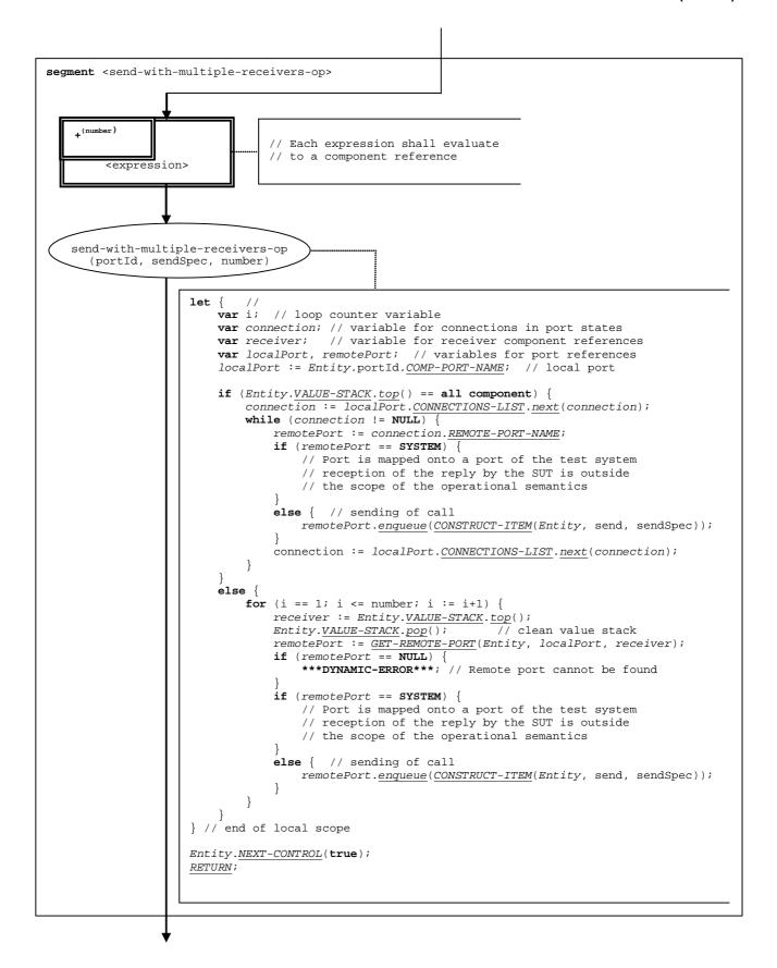
Figure 117a: Flow graph segment <send-with-multiple-receivers-op>
