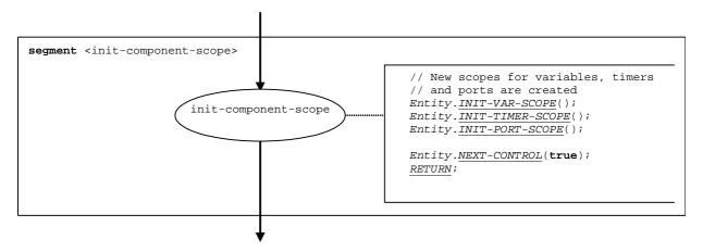
Figure 76: Flow graph segment <init-component-scope>
