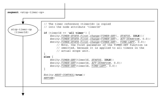
Figure 130: Flow graph segment <stop-timer-op>
