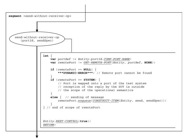
Figure 118: Flow graph segment <send-without-receiver-op>
