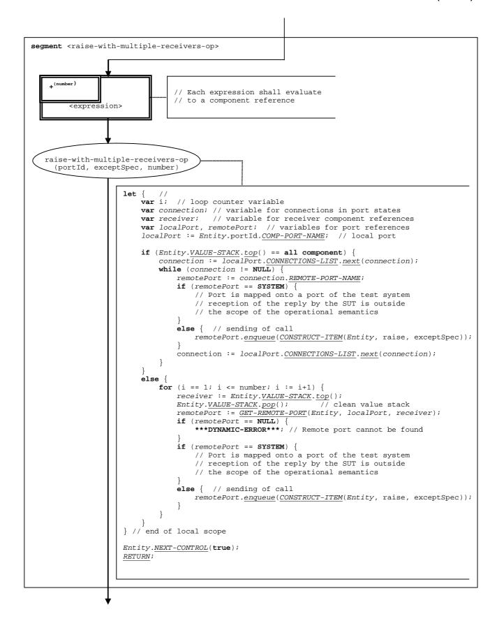
Figure 97a: Flow graph segment <raise-with-multiple-receivers-op>
