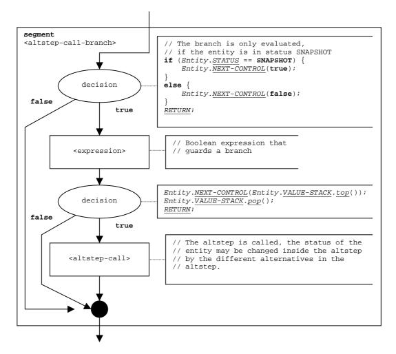
Figure 41: Flow graph segment <altstep-call-branch>
