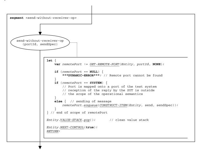
Figure 118: Flow graph segment <send-without-receiver-op>
