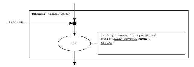
Figure 91: Flow graph segment < label-stmt>
