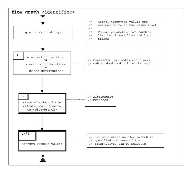
Figure 21: Flow graph representation of altsteps
