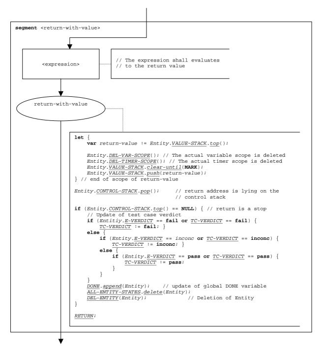
Figure 109: Flow graph segment <return-with-value>
