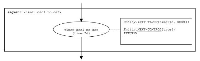
Figure 136: Flow graph segment <timer-decl-no-def>
