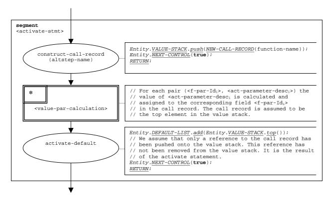
Figure 37: Flow graph segment <activate-stmt>
