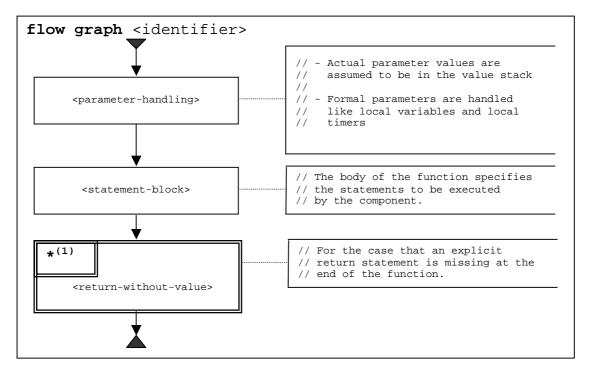
Figure 20: Flow graph representation of functions
