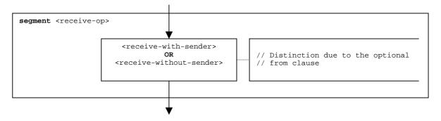
Figure 100: Flow graph segment <receive-op>
