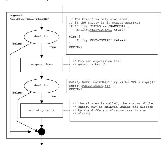
Figure 41: Flow graph segment <altstep-call-branch>
