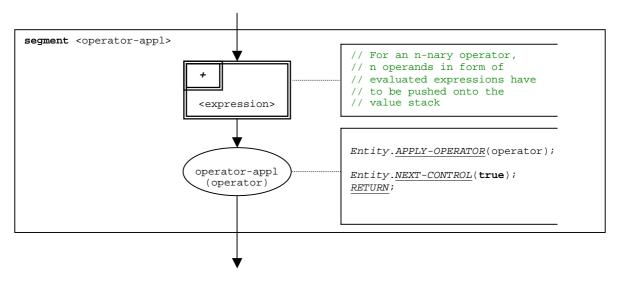
Figure 74: Flow graph segment < operator-appl>
