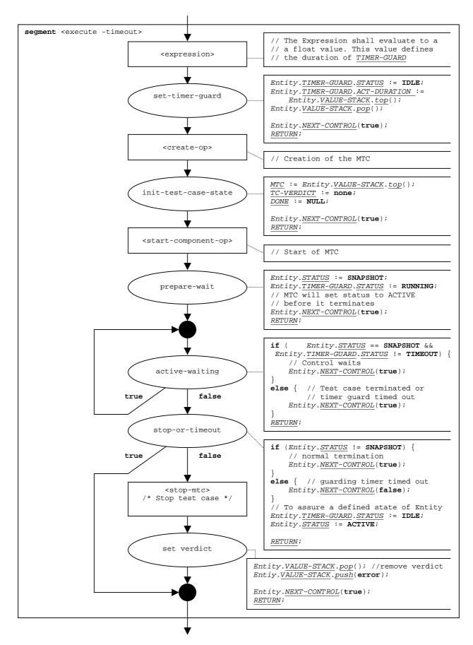
Figure 69: Flow graph segment <execute-timeout>
