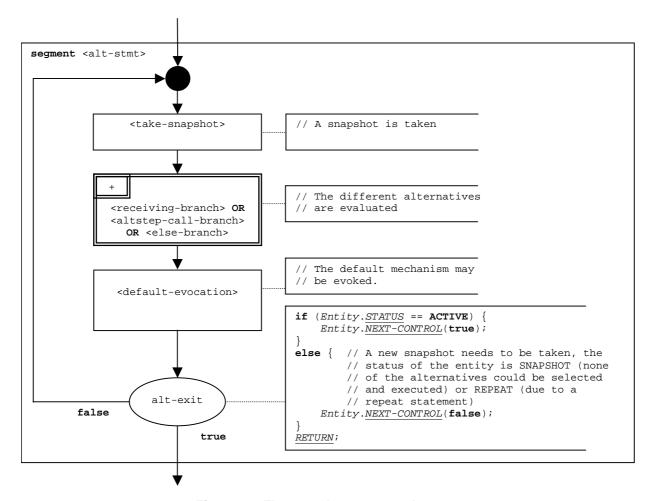
Figure 38: Flow graph segment <alt-stmt>
