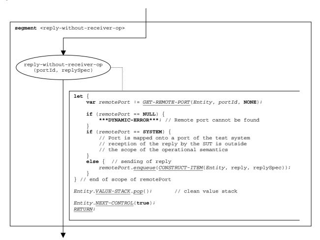
Figure 107: Flow graph segment <reply-without-receiver-op>
