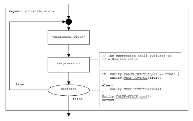
Figure 65: Flow graph segment <do-while-stmt>
