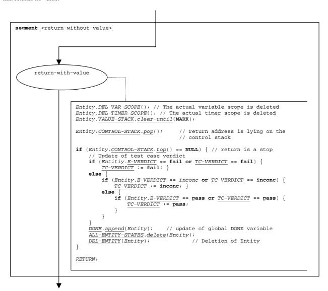
Figure 110: Flow graph segment <return-without-value>
