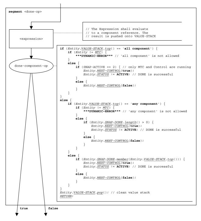
Figure 66: Flow graph segment <done-component-op>
