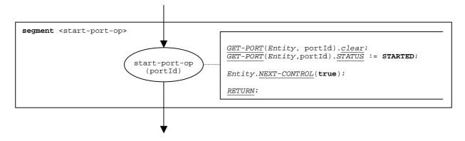
Figure 121: Flow graph segment <start-port-op>
