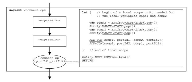
Figure 60: Flow graph segment <connect-op>
