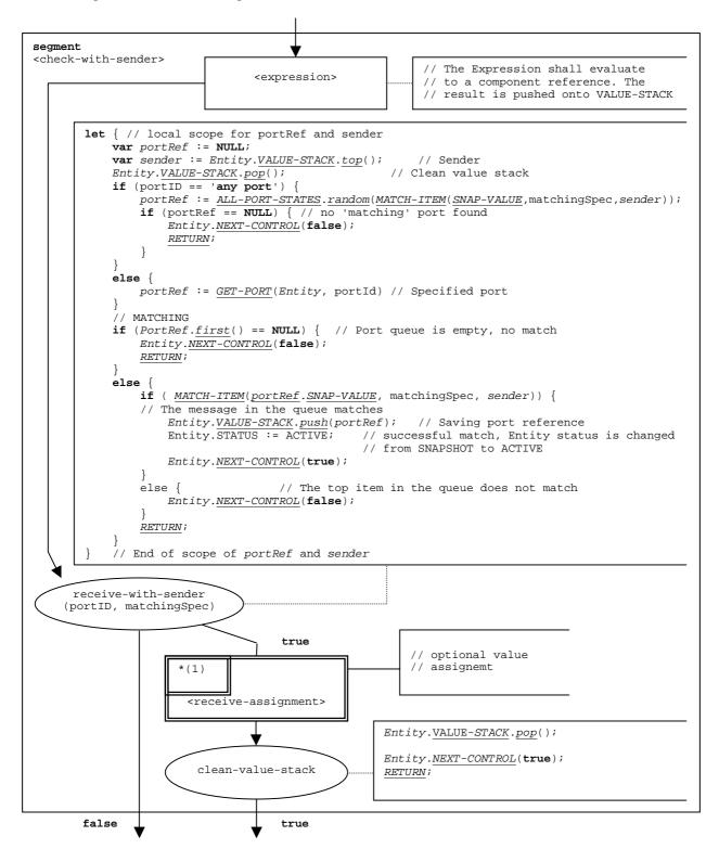
Figure 57: Flow graph segment <check-with-sender>
