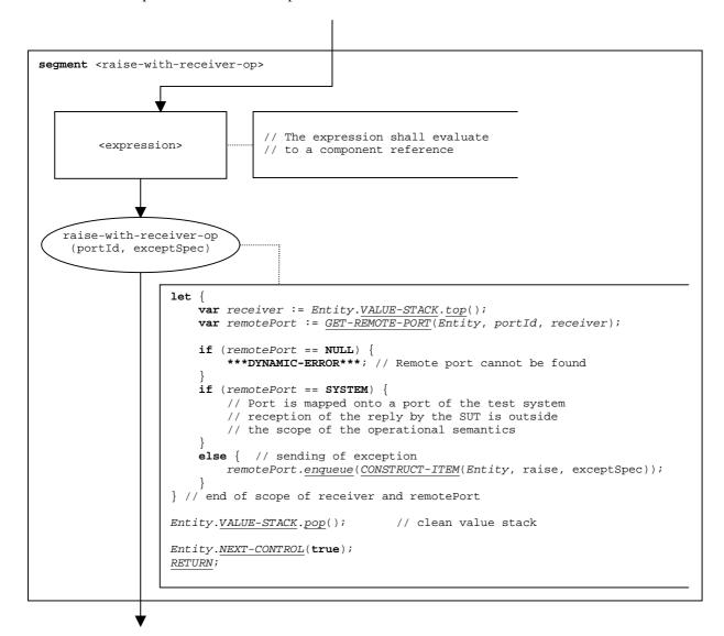
Figure 97: Flow graph segment <raise-with-receiver-op>
