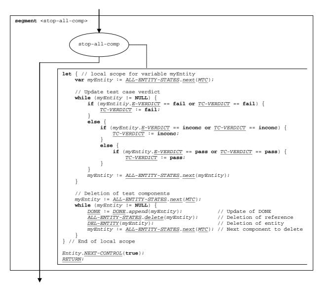
Figure 128: Flow graph segment <stop-all-comp>
