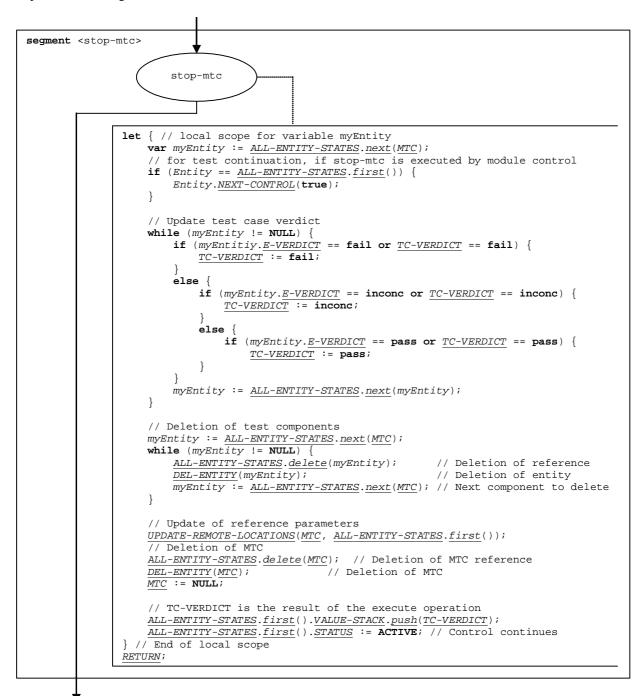
Figure 126: Flow graph segment <stop-mtc-op>
