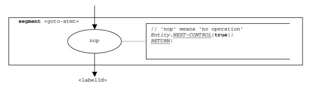
Figure 89: Flow graph segment <goto-stmt>
