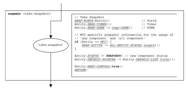
Figure 39: Flow graph segment <take-snapshot>
