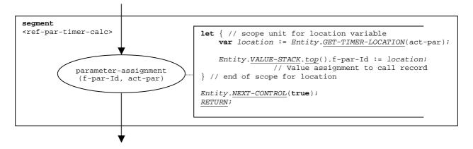
Figure 83: Flow graph segment <ref-par-timer-calc>
