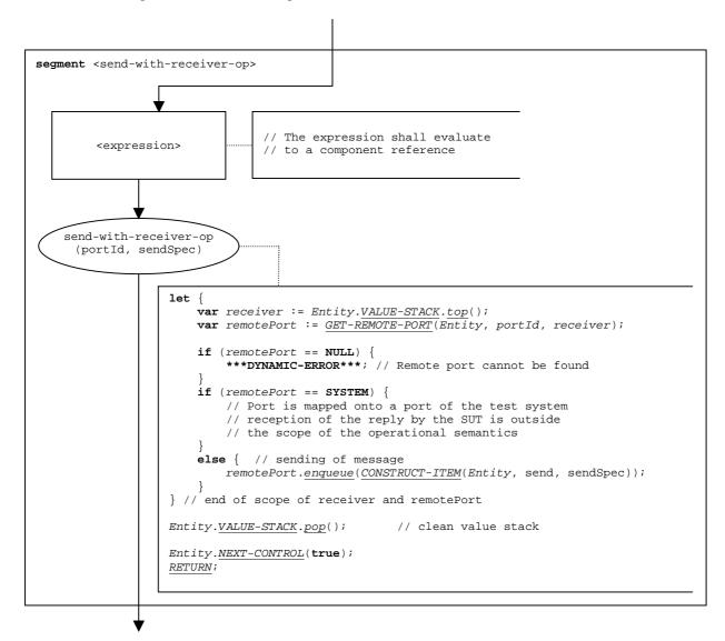
Figure 117: Flow graph segment <send-with-receiver-op>
