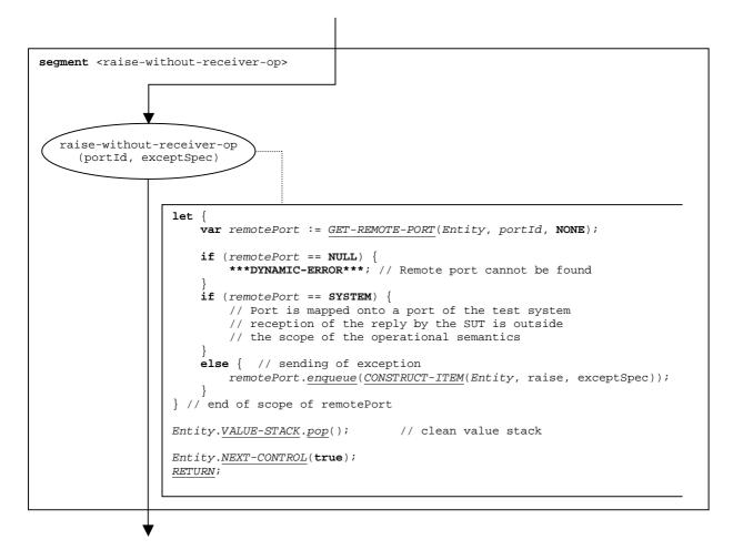
Figure 98: Flow graph segment <raise-without-receiver-op>
