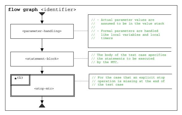
Figure 19: Flow graph representation of test cases
