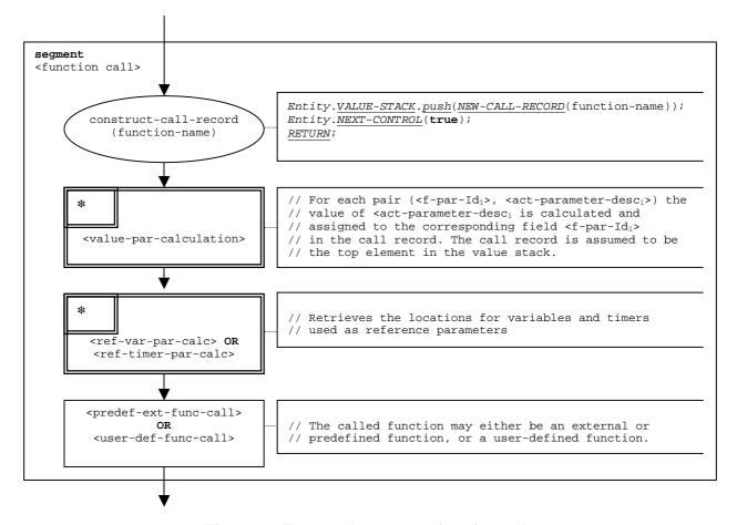
Figure 80: Flow graph segment <function-call>
