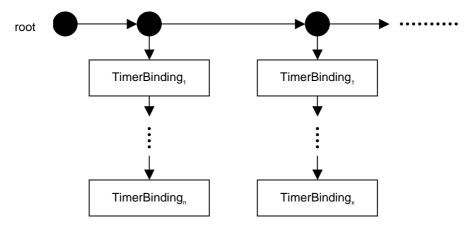
Figure 27: Structure of the <u>TIMER-STATE</u> part of an entity state
