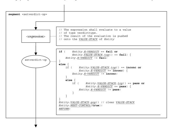
Figure 119: Flow graph segment <setverdict-op>
