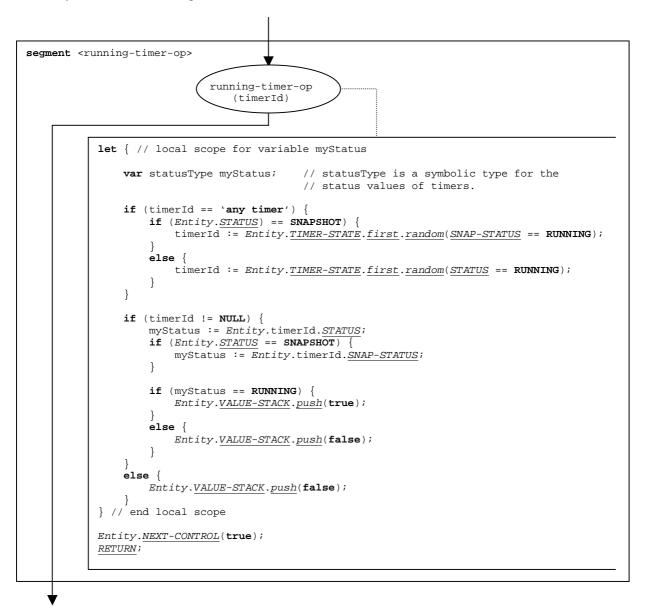
Figure 114: Flow graph segment <running-timer-op>
