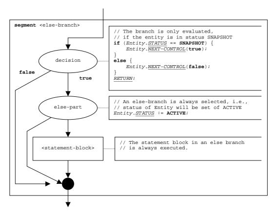
Figure 42: Flow graph segment <else-branch>
