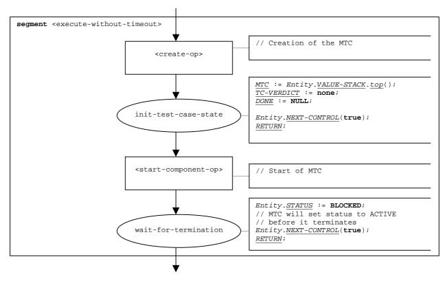
Figure 68: Flow graph segment <execute-without-timeout>
