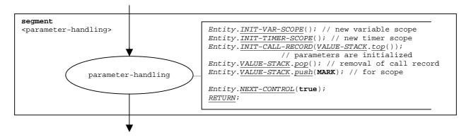
Figure 77: Flow graph segment cparameter-handling>
