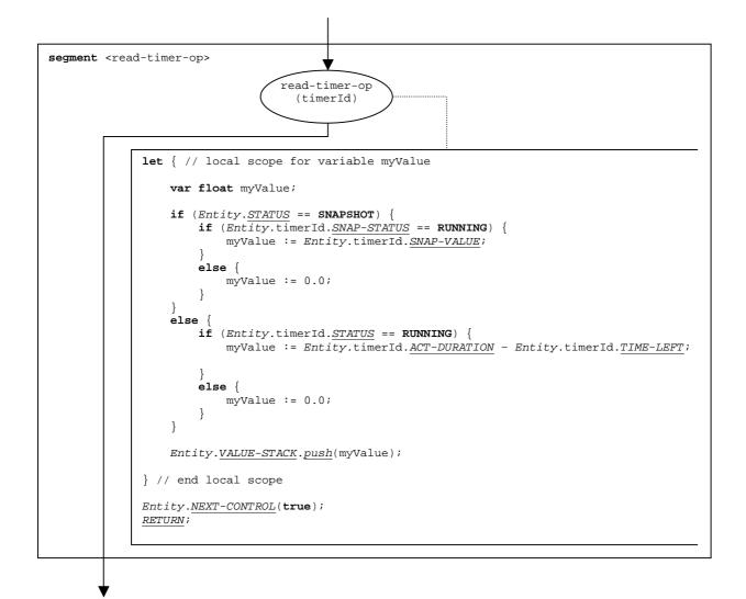
Figure 99: Flow graph segment <read-timer-op>
