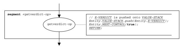
Figure 88: Flow graph segment <getverdict-op>
