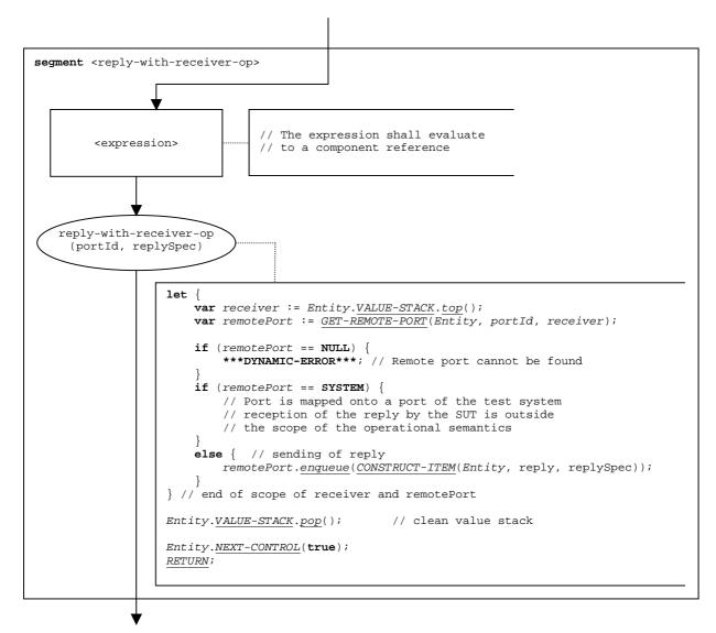
Figure 106: Flow graph segment <reply-with-receiver-op>
