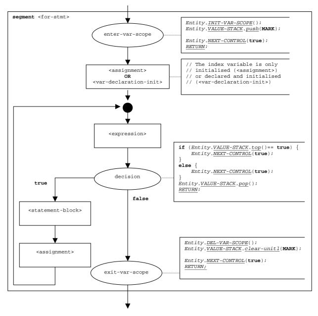
Figure 79: Flow graph segment <for-stmt>
