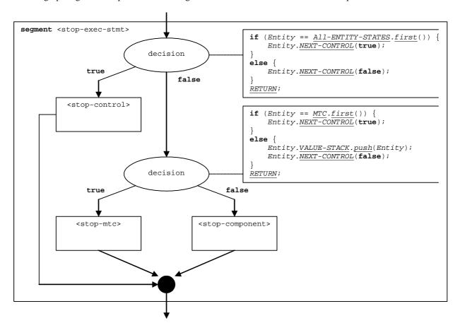
Figure 129: Flow graph segment <stop-exec-stmt>
