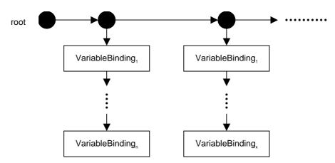
Figure 25: Structure of the **DATA-STATE** part of an entity state
