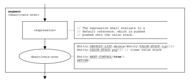
Figure 63: Flow graph segment <deactivate-stmt>
