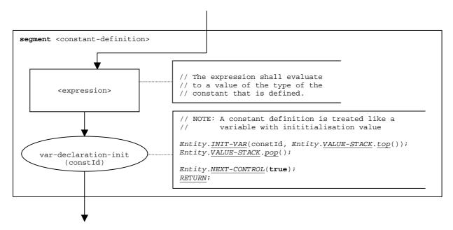
Figure 61: Flow graph segment <constant-definition>
