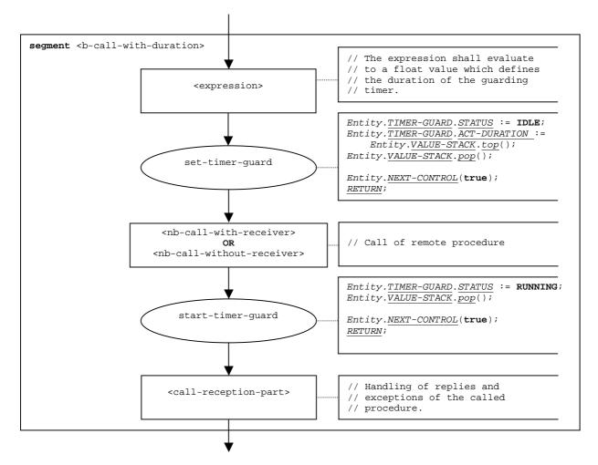
Figure 52: Flow graph segment <b-call-with-duration>
