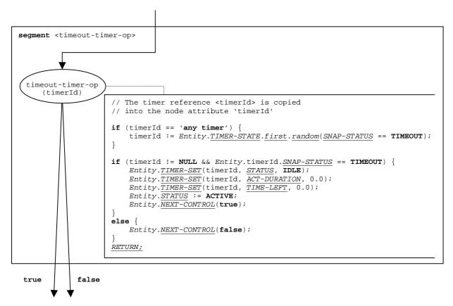
Figure 137: Flow graph segment <timeout-timer-op>
