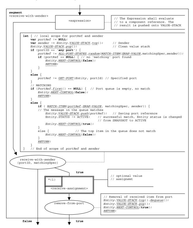
Figure 101: Flow graph segment <receive-with-sender>
