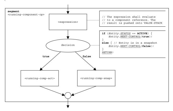
Figure 111: Flow graph segment <running-component-op>
