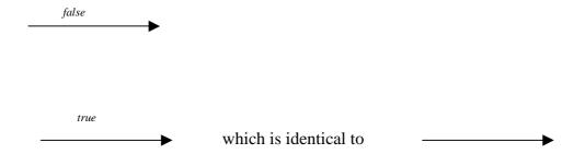
To support the joining of several flow lines into one flow line on a graphical level, a special join node is introduced. The join node and an example for its usage are shown below:
