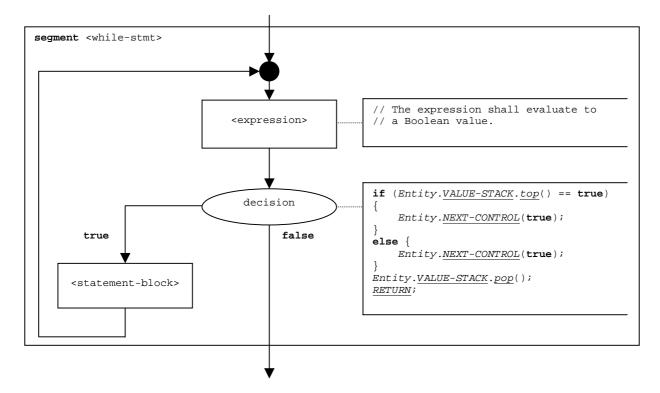
Figure 140: Flow graph segment <while-stmt>
