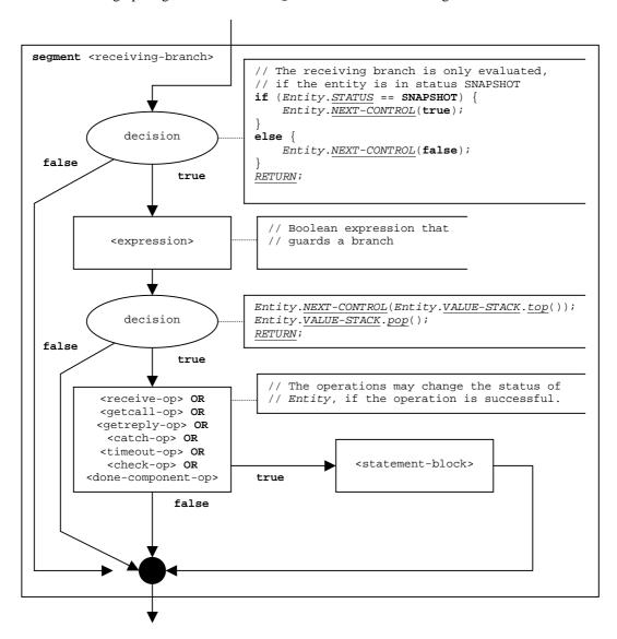
Figure 40: Flow graph segment <receiving-branch>
