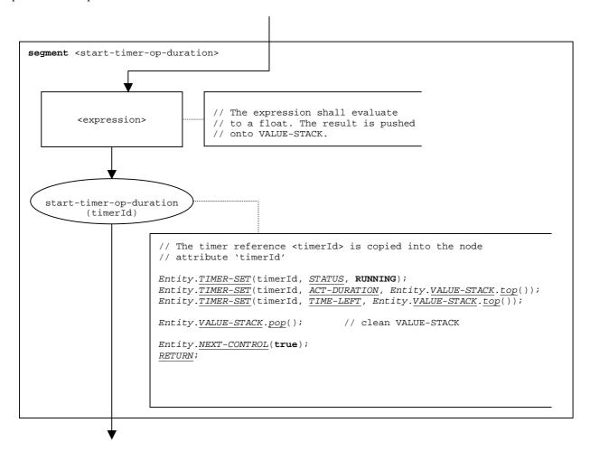
Figure 124: Flow graph segment <start-timer-op-duration>
