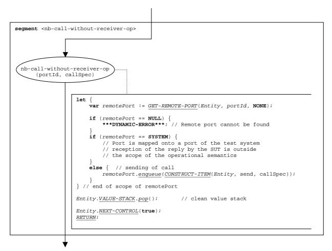
Figure 50: Flow graph segment <nb-call-without-receiver>
