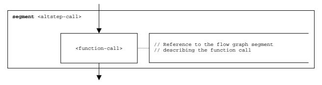
Figure 44: Flow graph segment <altstep-call>
