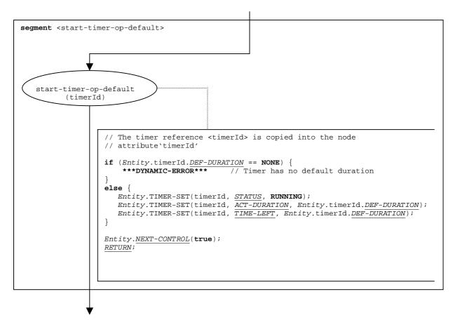
Figure 123: Flow graph segment <start-timer-op-default>
