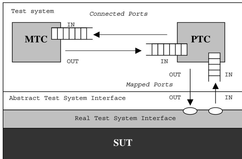
Figure 10: Illustration of the connect and map operations
