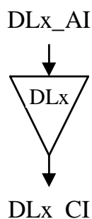
Figure 17: SDI Data Link type x Trail Termination Source (DLx_TT_So)
