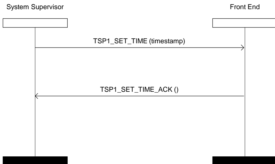
Figure 9: Example of normal operation of the TSP1_SET_TIME PDU
