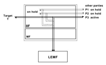
Figure A.5.2: CC link option B (example for call hold supplementary service)
