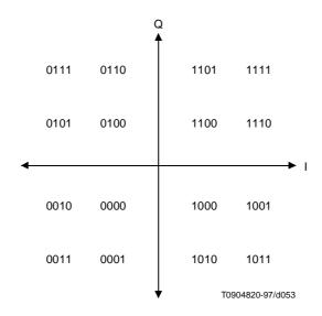
Figure N-3: 16QAM differential-coded symbol mapping
