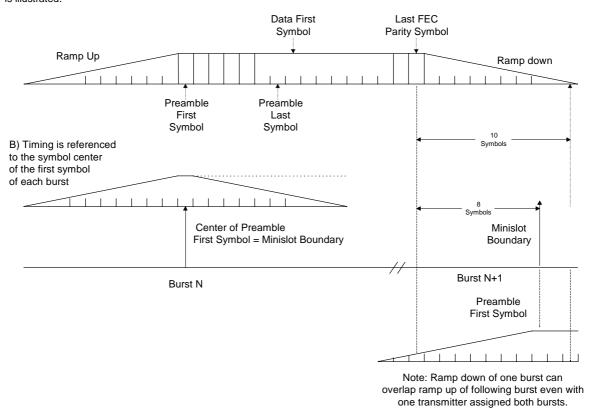
Figure 6-6: Nominal Burst Timing
