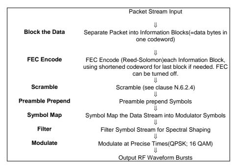
Figure N-10: TDMA upstream transmission processing
