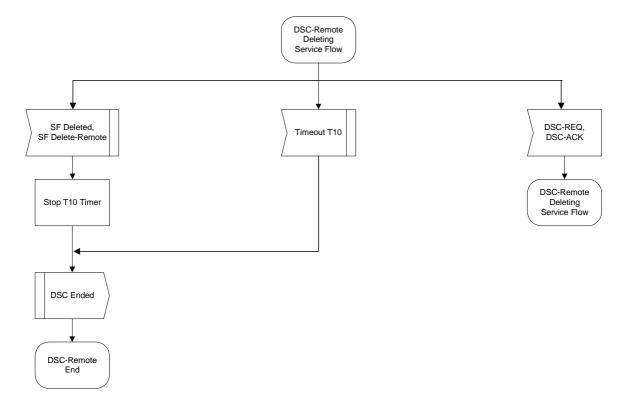
Figure 11-49: DSC-Remotely Initiated Transaction Deleting Service Flow State Flow Diagram
