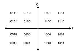
Figure 6-3: 16QAM Differential-Coded Symbol Mapping
