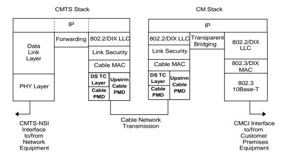
Figure 5-2: Data Forwarding Through the CM and CMTS
