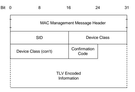
Figure 8-43: Device Class Identification Response
