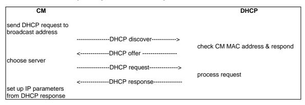
Figure 11-10: Establishing IP Connectivity
