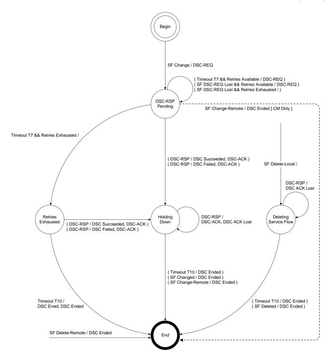
Figure 11-24: DSC-Locally Initiated Transaction State Transition Diagram
