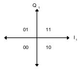
Figure 6-1: QPSK Symbol Mapping
