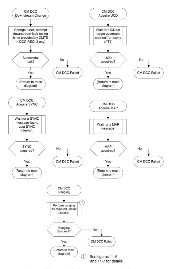
Figure 11-64: Dynamically Changing Channels: CM View Part 3
