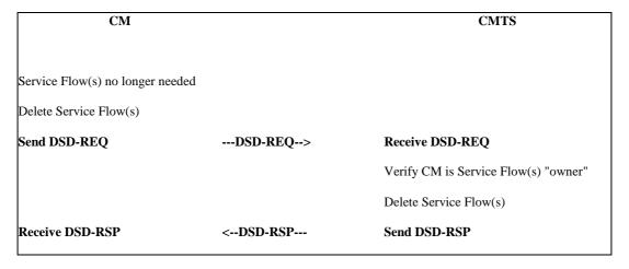
Figure 11-50: Dynamic Service Deletion Initiated from CM
