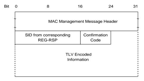
Figure 8-28: Registration Acknowledgment
