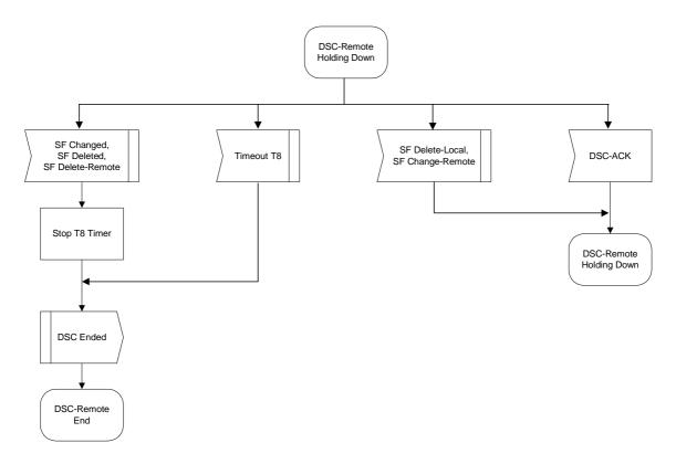
Figure 11-48: DSC-Remotely Initiated Transaction Holding Down State Flow Diagram
