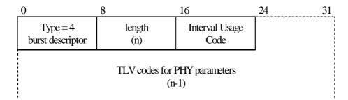
Figure 8-17: Top-Level Encoding for a Burst Descriptor
