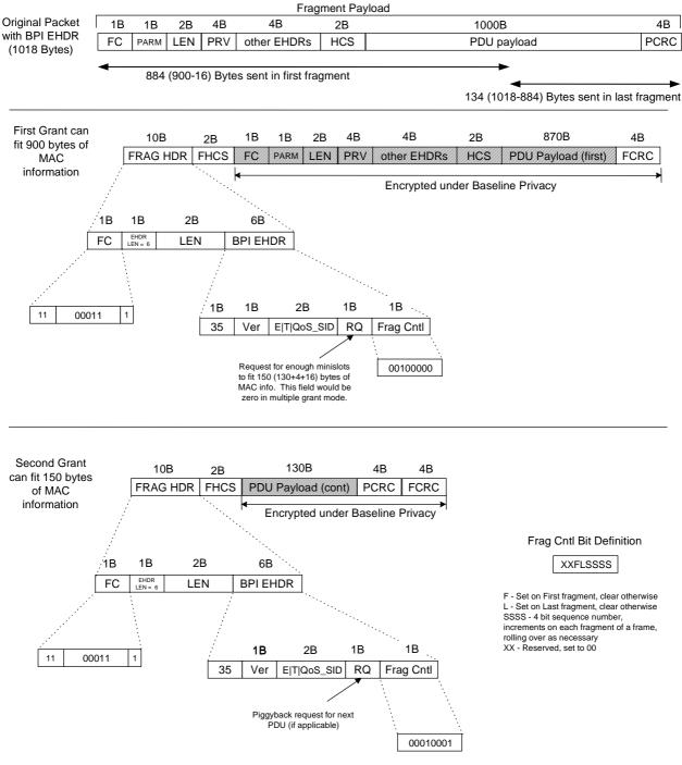
Figure 10-9: Example of Fragmenting a Single Packet
