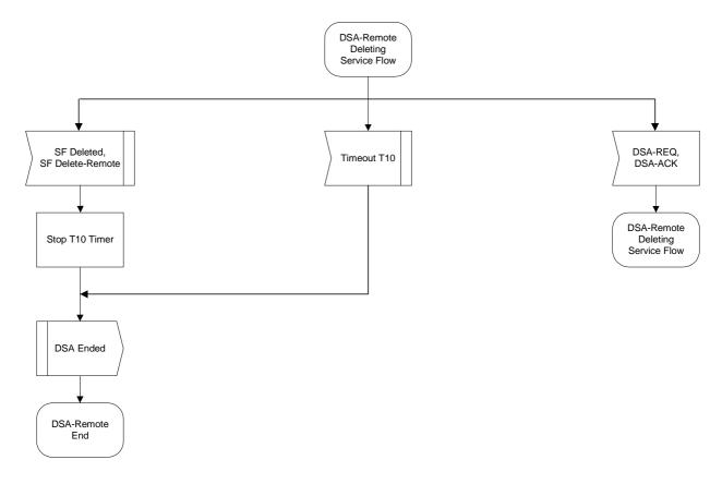
Figure 11-38: DSA-Remotely Initiated Transaction Deleting Service State Flow Diagram
