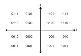
Figure 6-2: 16QAM Gray-Coded Symbol Mapping
