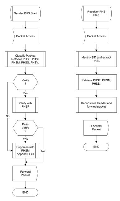
Figure 10-11: Payload Header Suppression Operation
