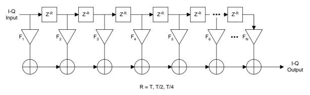
Figure N-5: Transmit Pre-Equalizer Structure
