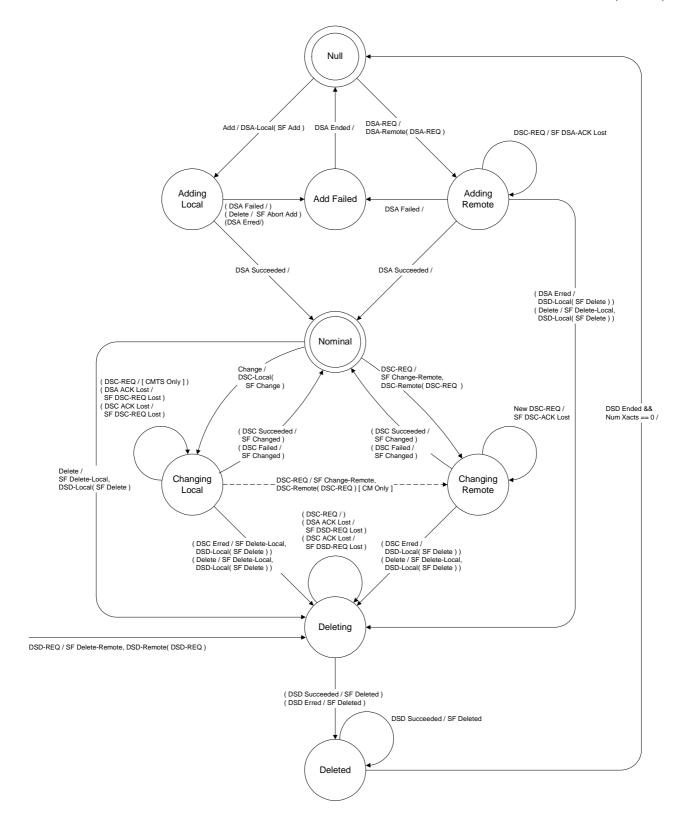
Figure 11-21: Dynamic Service Flow State Transition Diagram
