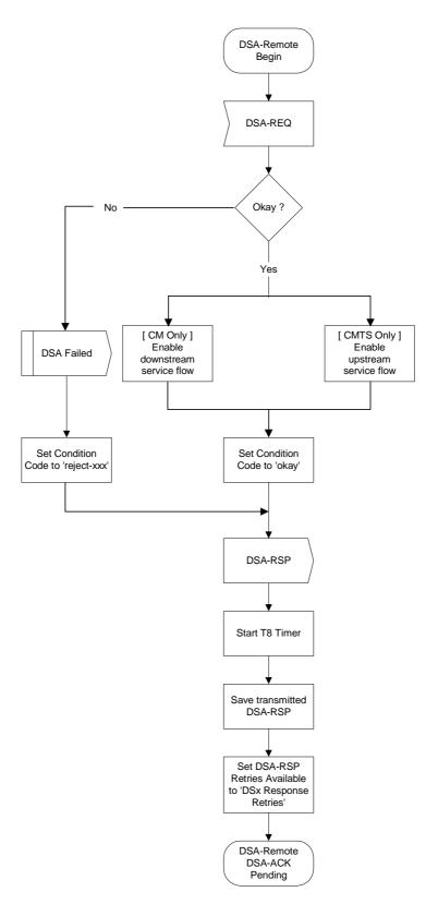
Figure 11-35: DSA-Remotely Initiated Transaction Begin State Flow Diagram
