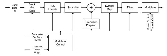
Figure N-9: Signal-processing sequence
