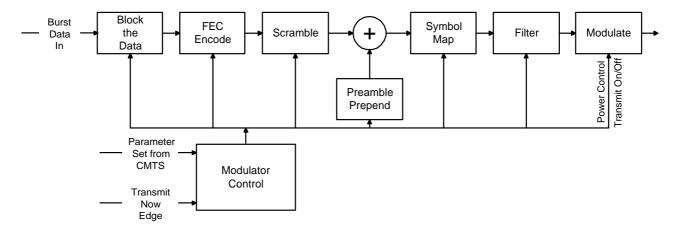
Figure 6-9: Signal-Processing Sequence
