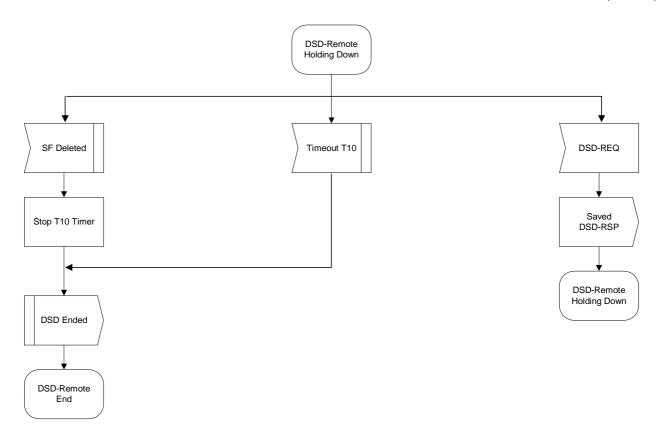
Figure 11-56: DSD-Remotely Initiated Transaction Holding Down State Flow Diagram
