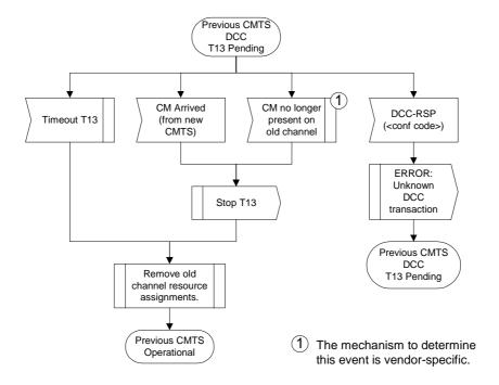
Figure 11-60: Dynamically Changing Channels: CMTS View Part 3
