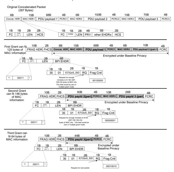
Figure 10-10: Fragmented Concatenated Packet Example
