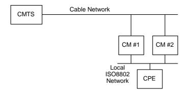
Figure 5-3: Example Condition for Network Loops
