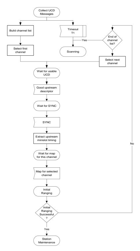
Figure 11-3: Obtaining Upstream Parameters
