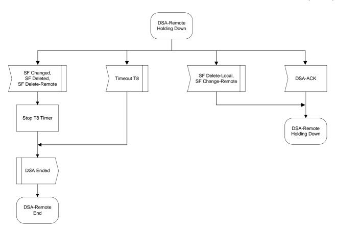
Figure 11-37: DSA-Remotely Initiated Transaction Holding Down State Flow Diagram
