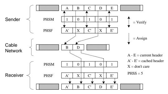
Figure 10-12: Payload Header Suppression with Masking
