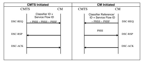
Figure 10-13: Payload Header Suppression Signalling Example
