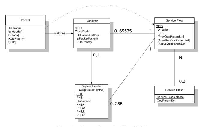
Figure 10-4: Theory of Operation Object Model
