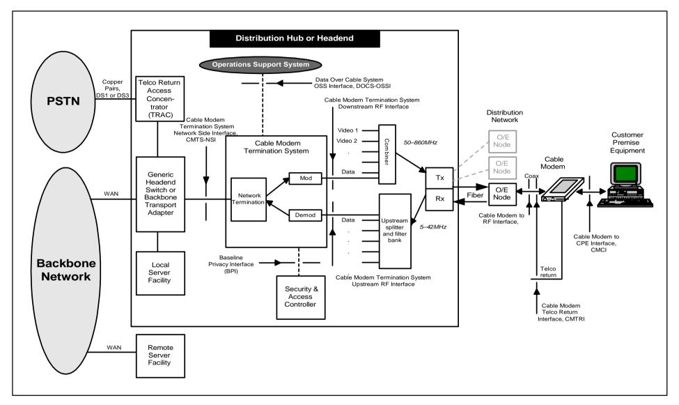
Figure 1-2: Data-Over-Cable Reference Architecture
