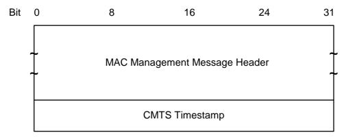
Figure 8-15: Format of Packet PDU Following the Timing Header
