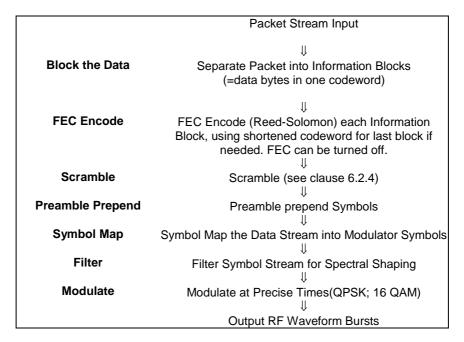
Figure 6-10: TDMA Upstream Transmission Processing
