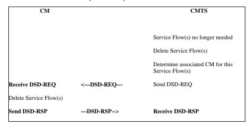
Figure 11-51: Dynamic Service Deletion Initiated from CMTS
