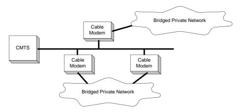
Figure I-1: Spanning Tree Topology
