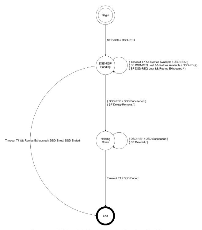
Figure 11-26: DSD-Locally Initiated Transaction State Transition Diagram
