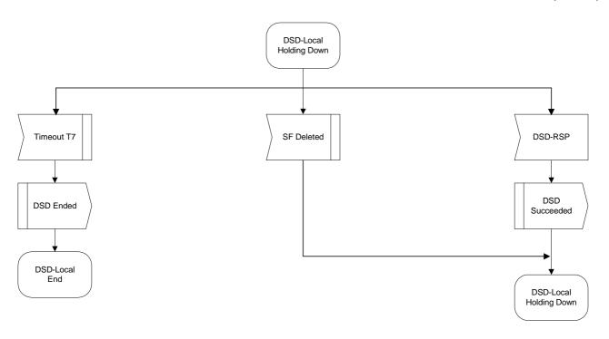
Figure 11-54: DSD-Locally Initiated Transaction Holding Down State Flow Diagram
