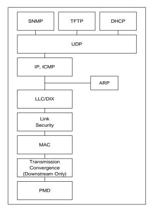
Figure 5-1: Protocol Stack on the RF Interface
