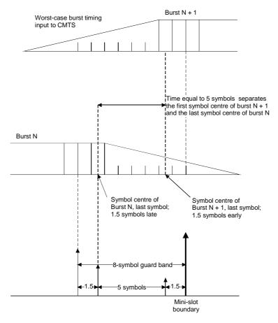
Figure N-7: Worst-case burst timing
