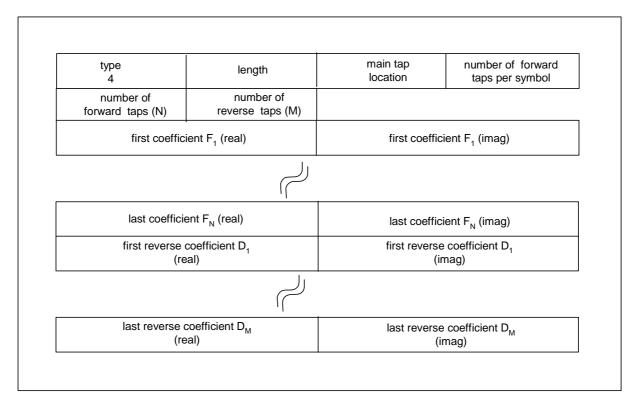
Figure 8-23: Generalized Decision Feedback Equalization Coefficients
