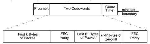
Figure 6-8: Example Frame Structures with Flexible Burst Length Mode
