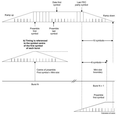
NOTE-Ramp down of one burst can overlap ramp up of following burst even with one transmitter assigned both bursts.
