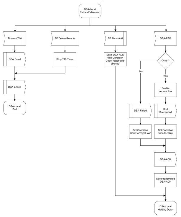
Figure 11-33: DSA-Locally Initiated Transaction Retries Exhausted
