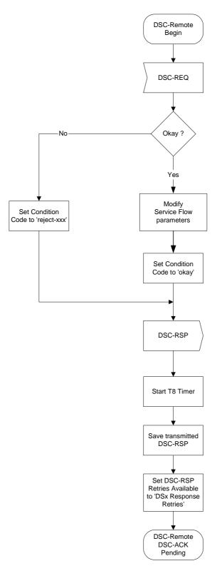
Figure 11-46: DSC-Remotely Initiated Transaction Begin State Flow Diagram
