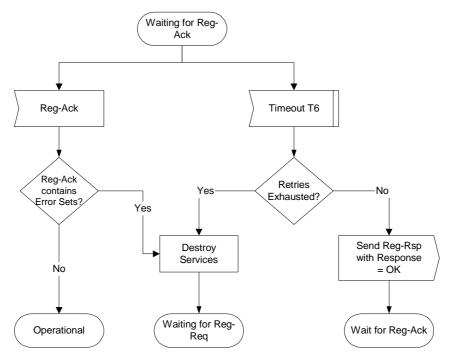
Figure 11-15: Registration Acknowledgment- CMTS
