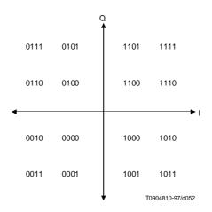
Figure N-2: 16QAM Gray-coded Symbol Mapping
