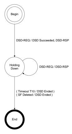
Figure 11-27: Dynamic Deletion (DSD) - Remotely Initiated Transaction State Transition Diagram
