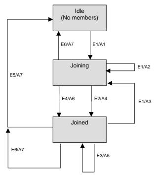
Figure L-1: IGMP Support - CM passive mode
