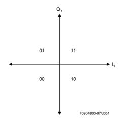
Figure N-1: QPSK Symbol Mapping
