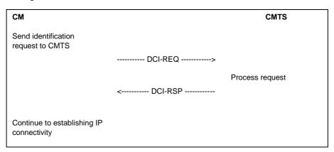
Figure 11-9: Device Class Identification
