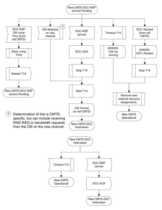
Figure 11-61: Dynamically Changing Channels: CMTS View Part 4
