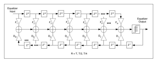
Figure 8-24: Generalized Equalizer Tap Location Definition
