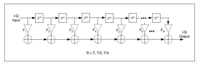
Figure 6-5: Transmit Pre-Equalizer Structure
