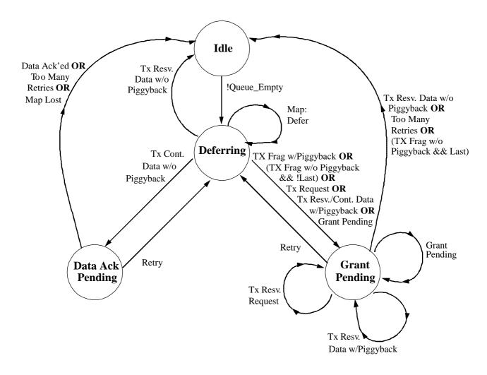
Figure K-1: Transmission & Deference State Transition Diagram
