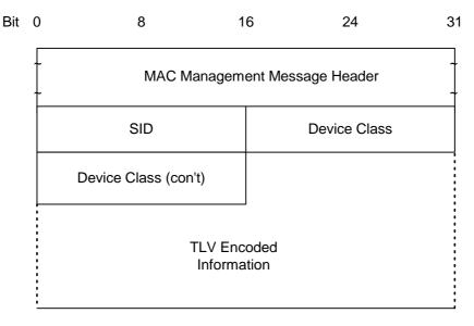
Figure 8-42: Device Class Identification Request
