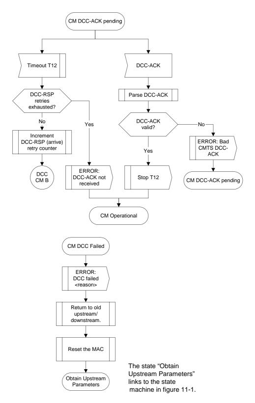
Figure 11-65: Dynamically Changing Channels: CM View Part 4
