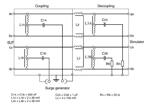
NOTE: L2 shall be a 4-coil current compensated choke to avoid saturation of coils due to phantom power feeding.
