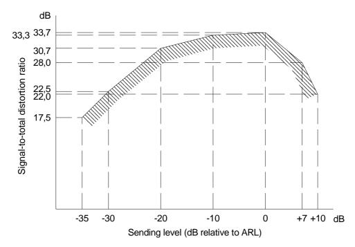
Figure 17: Limits for signal-to-distortion ratio, sending, method 2
