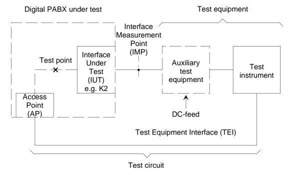
Figure A.1: Basic measurement configuration
