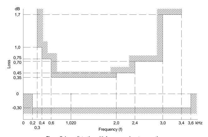
Figure 7: Loss distortion with frequency - input connection
