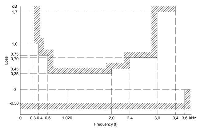
Figure 8: Loss distortion with frequency - output connection
