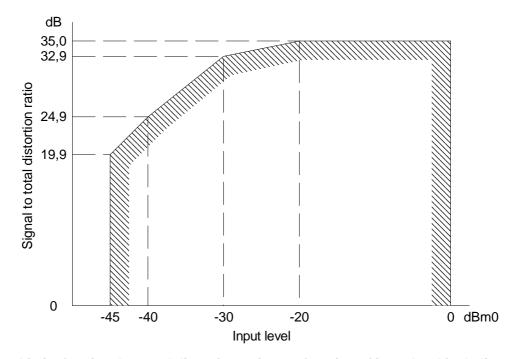
Figure 11: Limits for signal-to-total distortion ratio as a function of input level including analogue noise. Input connection ( $L_i = 0$  dBr). Interfaces L2 and M2 with feeding bridges
