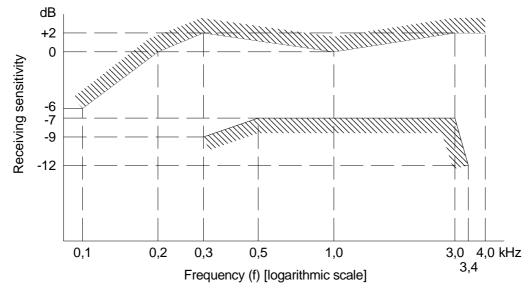
Figure 15: Receive sensitivity/frequency mask
