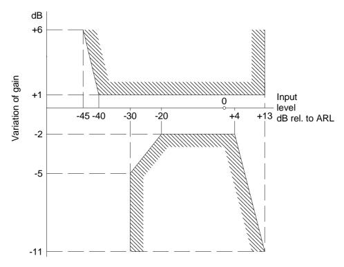
Figure 20: Variation of gain with input level (sending)
