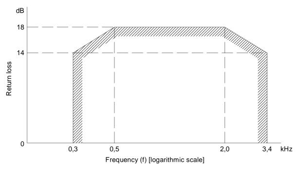
Figure 5: Minimum value of return loss against the nominal PBX impedance
