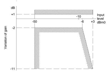
Figure 21: Variation of gain with input level (receiving)
