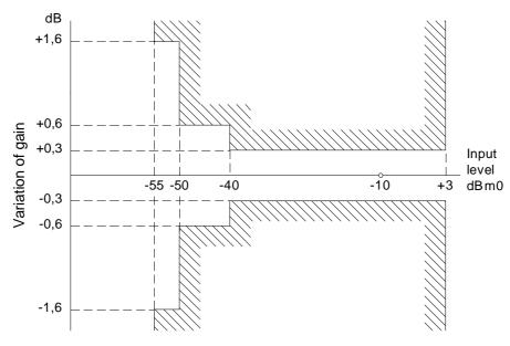
Figure 6: Variation of gain with input level
