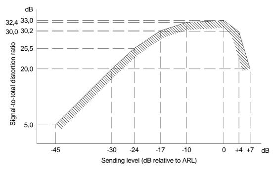
Figure 16: Limits of signal-to-distortion ratio, sending, method 1
