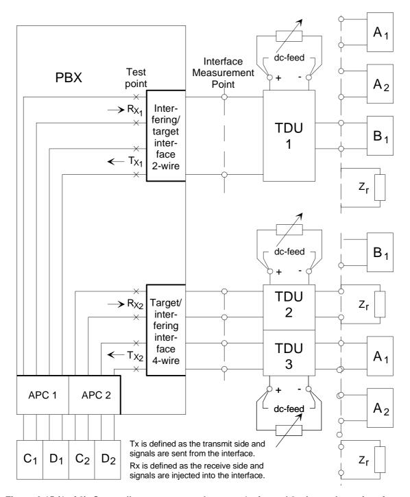
Figure A.15 (1 of 2): Crosstalk measurements between 4-wire and 2-wire analogue interfaces
