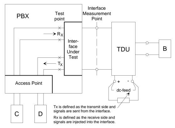
Figure A.8: 2-wire analogue interface, output connection
