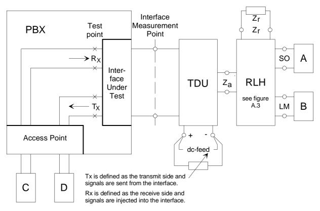
Figure A.10: 2-wire analogue interface, return loss
