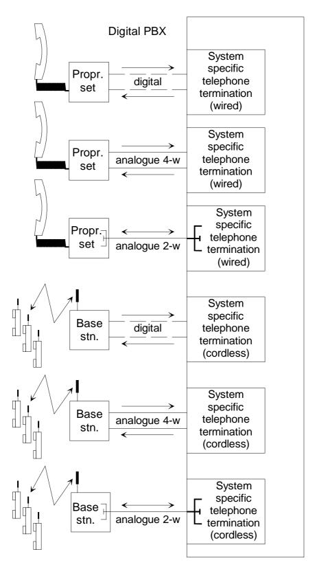
Figure 4: System specific telephone configurations (wired or cordless)
