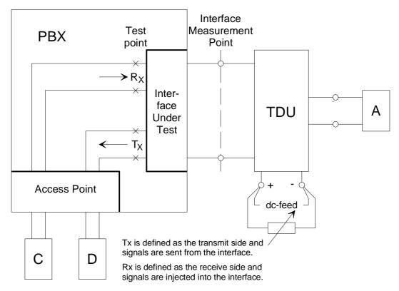
Figure A.6: 2-wire analogue interface, input connection
