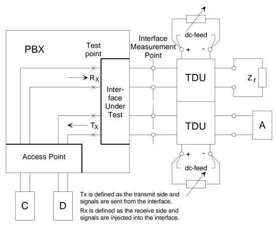
Figure A.7: 4-wire analogue interface, input connection
