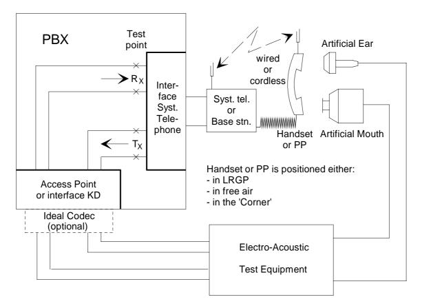
Figure A.20: Test configuration for electro-acoustic measurements
