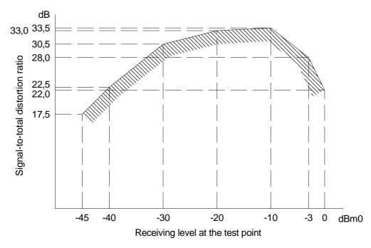
Figure 19: Limits for signal-to-distortion ratio, receiving, method 2
