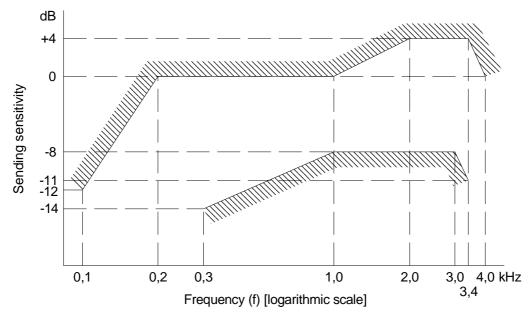
Figure 14: Send sensitivity/frequency mask
