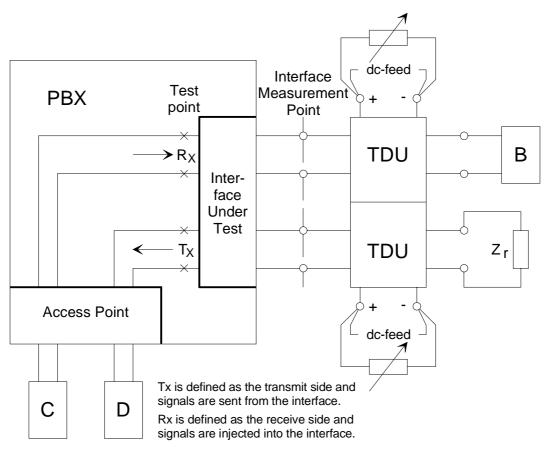
Figure A.9: 4-wire analogue interface, output connection
