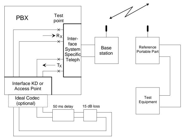
Figure A.23: Test configuration for measurement of Talker Echo Loudness Rating (case 3)
