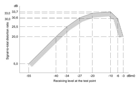
Figure 18: Limits of signal-to-distortion ratio, receiving, method 1
