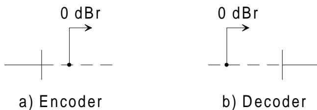
**Figure D.6: 0 dBm level reference points for codecs**
