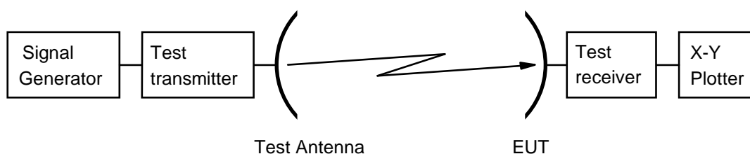
Figure 9: Test arrangement - antenna transmit radiation pattern measurement
