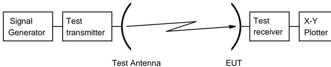
Figure 9: Test arrangement - antenna transmit radiation pattern measurement
