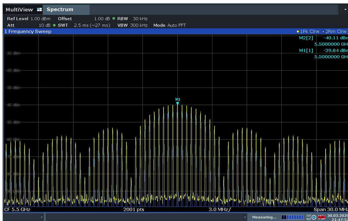
Figure F.6: Max and mean PSD of a pulse train line spectrum
