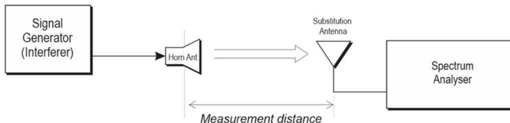
**Figure C.3: Measurement set up for calibration**
