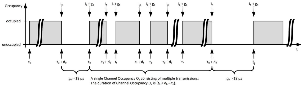
**Figure 9: Example of UUT transmissions**
