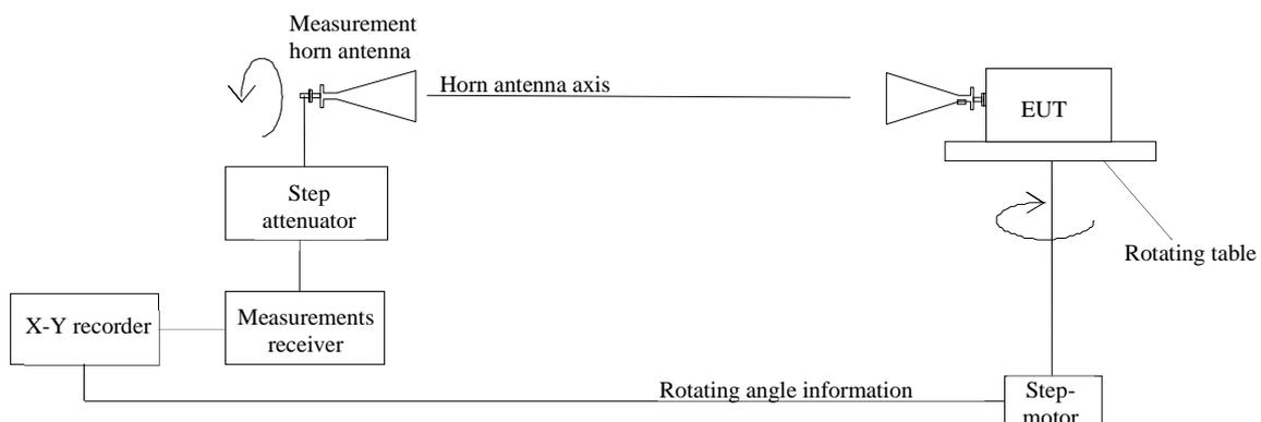
**Figure 13: Test set-up for measurement of antenna pattern**
