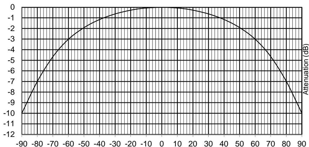
Figure 5: Minimum attenuation of the horizontal antenna pattern
