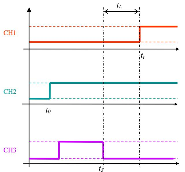
**Figure 10: Minimum listen time after detection,  $t_L$ , measurement**
