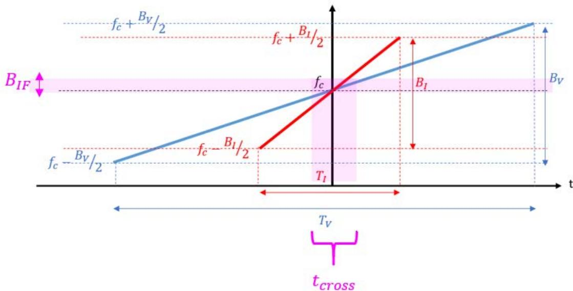
Figure E.2: Crossing time  $t_{cross}$  between interfering signals
