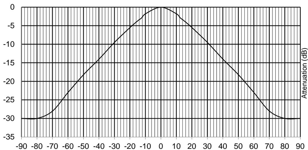
Figure 4: Minimum attenuation of the vertical antenna pattern
