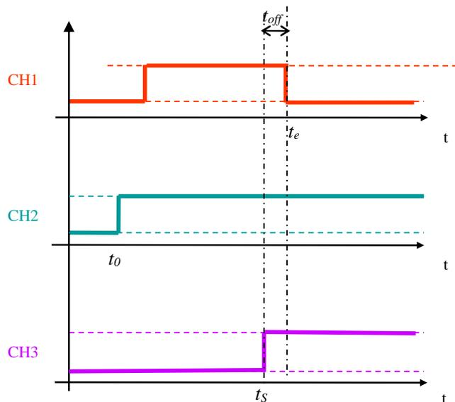
Figure 11: Maximum transmit switch-off time,  $t_{off}$  measurement
