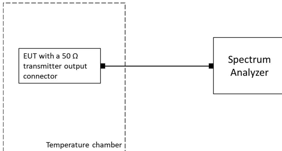
**Figure 6: Setup for conducted measurements**
