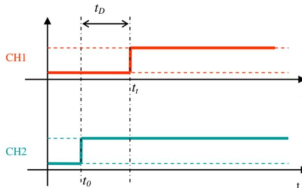
Figure 9: Minimum listen time,  $t_D$ , measurement
