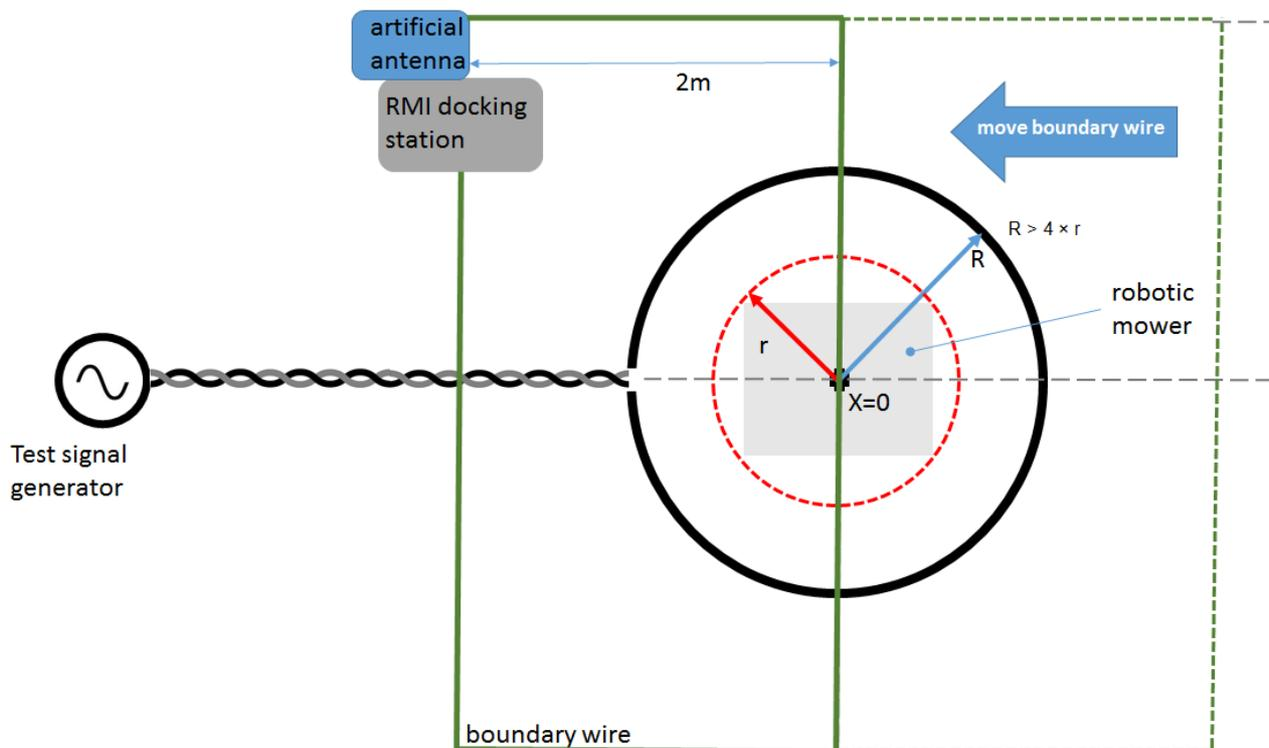
Figure 6: Schematic test set-up for the RX-blocking test 2
