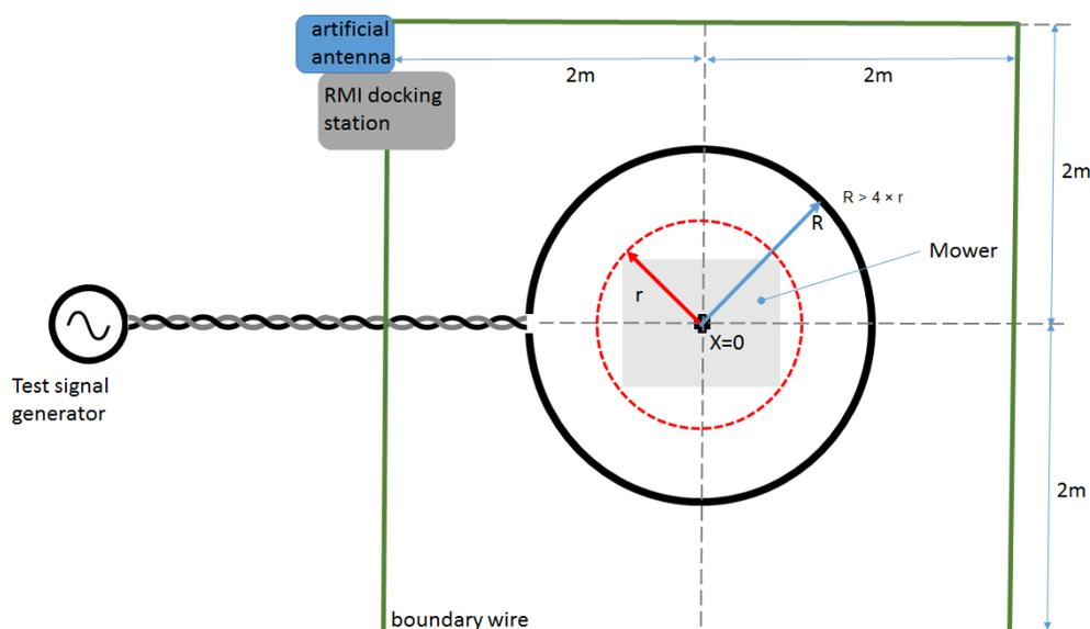
Figure 5: Schematic test set-up for the RX-blocking test 1
