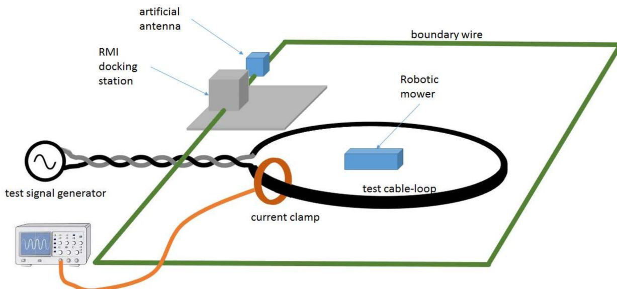
Figure 4: Schematic test set-up for the RX-blocking test 1
