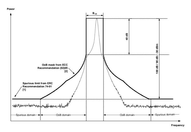
Figure 3: Definition of OoB and spurious emission domains for non FM/PM pulsed radar (Not to scale)
