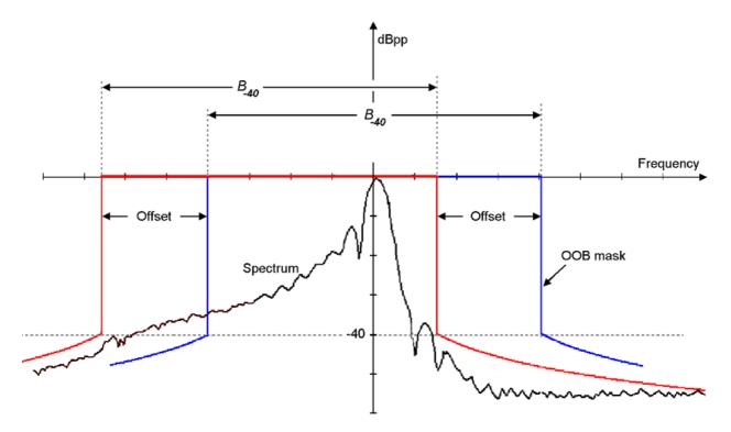
Figure B.1: Application of the offset-rule for the OoB emission limit mask
