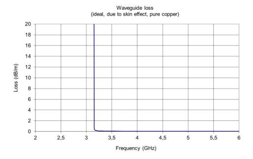
Figure G.1: attenuation for an ideal waveguide
