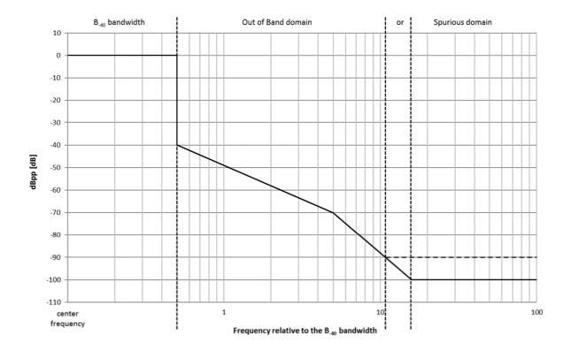
Figure 2: Unwanted emission limit masks
