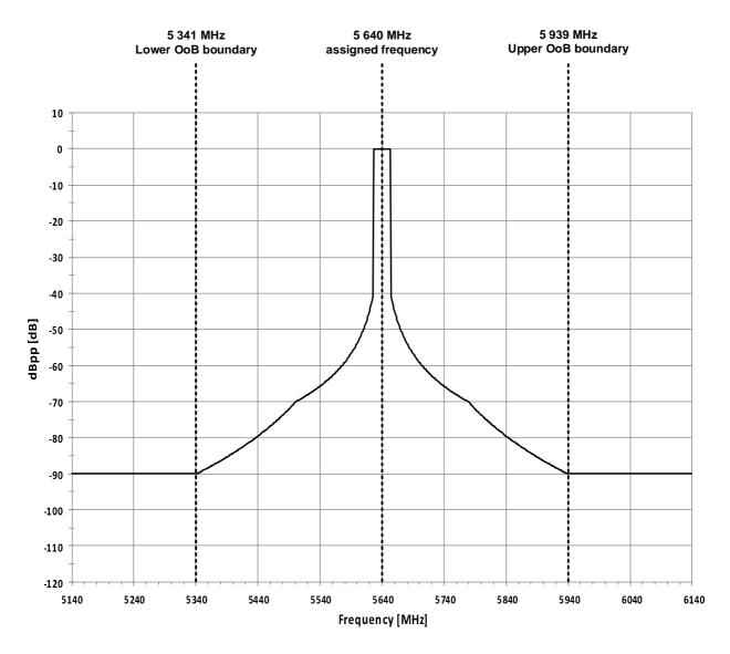
Figure 7: Example of a calculated emissions mask for pulse duration t = 500 ns and rise time  $t_r$  = 100 ns at centre frequency of 5 640 MHz
