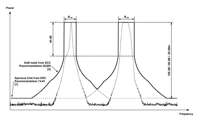
Figure 1: Example of superimposed (combined) mask from two carrier frequencies
