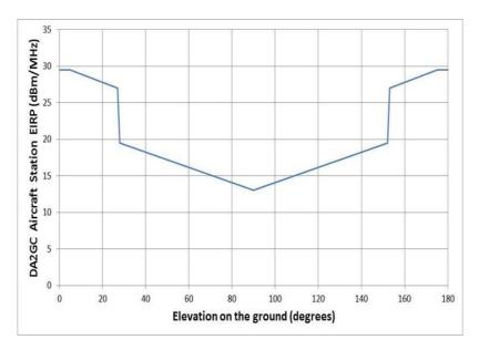
Figure 2: Example of AS EIRP mask for an aircraft height above ground of 10 km
