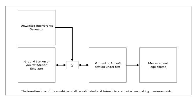
Figure B.1: Measurement system for receiver ACS
