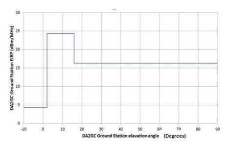
Figure 1: EIRP mask as a function of elevation angle for the Ground Station
