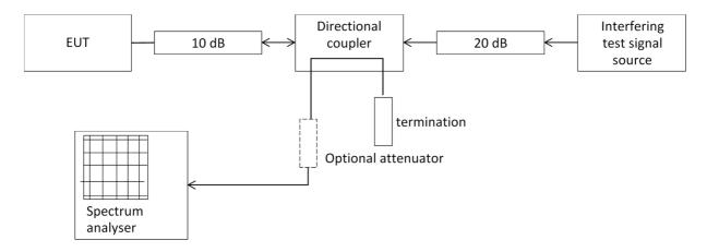
Figure 4: Measurement Arrangement
