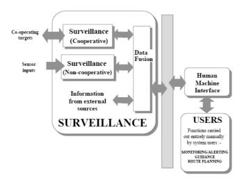
Figure 1: A-SMGCS Level 1 Functional Configuration
