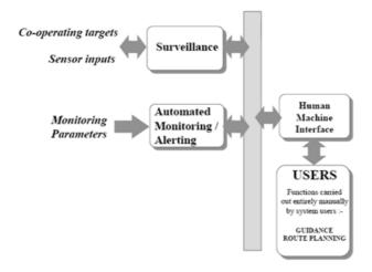
Figure 2: A-SMGCS Level 2 Functional Configuration
