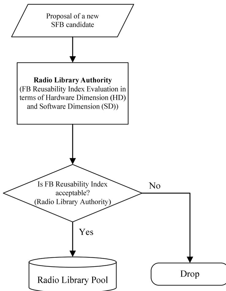
**Figure D.1: Flow chart for determining SFBs**
