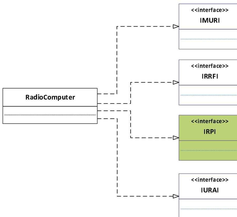
**Figure 4.2: UML® class diagram for Radio Computer interfaces**
