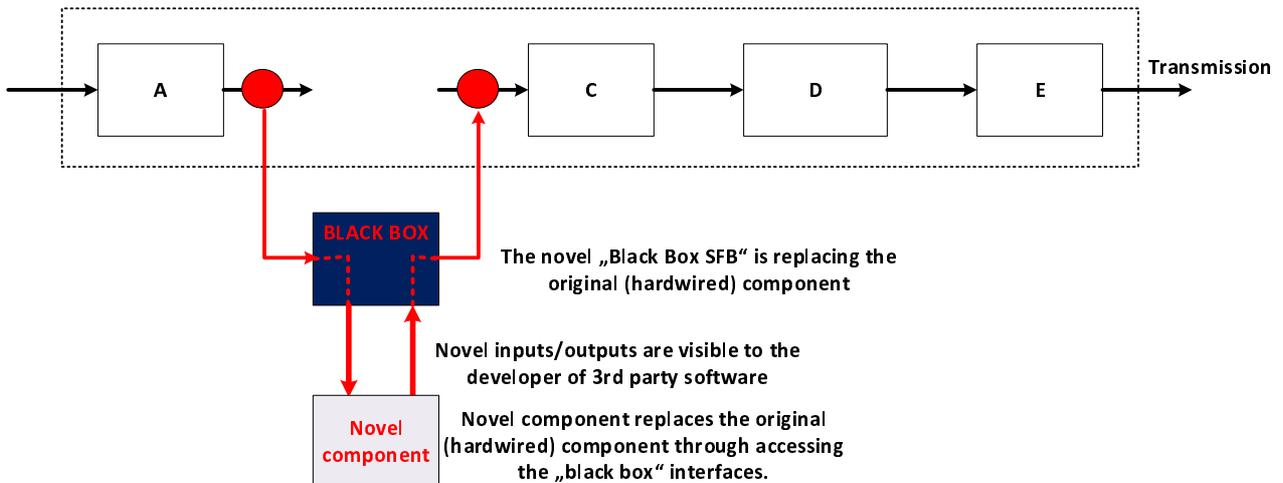
**Figure C.2: Example replacement of a component through interfacing with novel SFB provided by a (3<sup>rd</sup> party) software provider**
