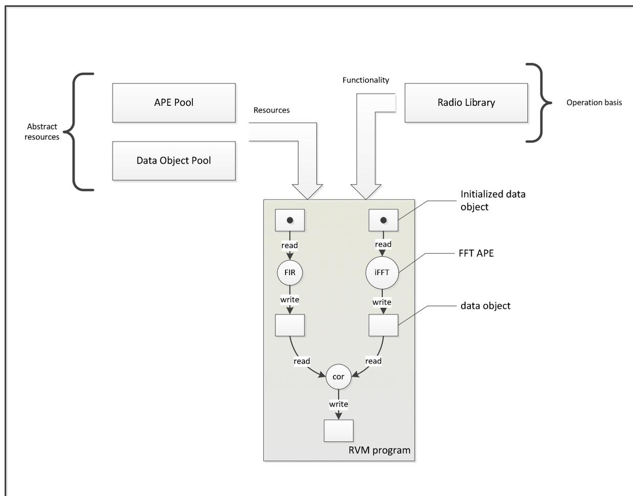
Figure 6.1: Conceptual Diagram of Radio Virtual Machine Processing
