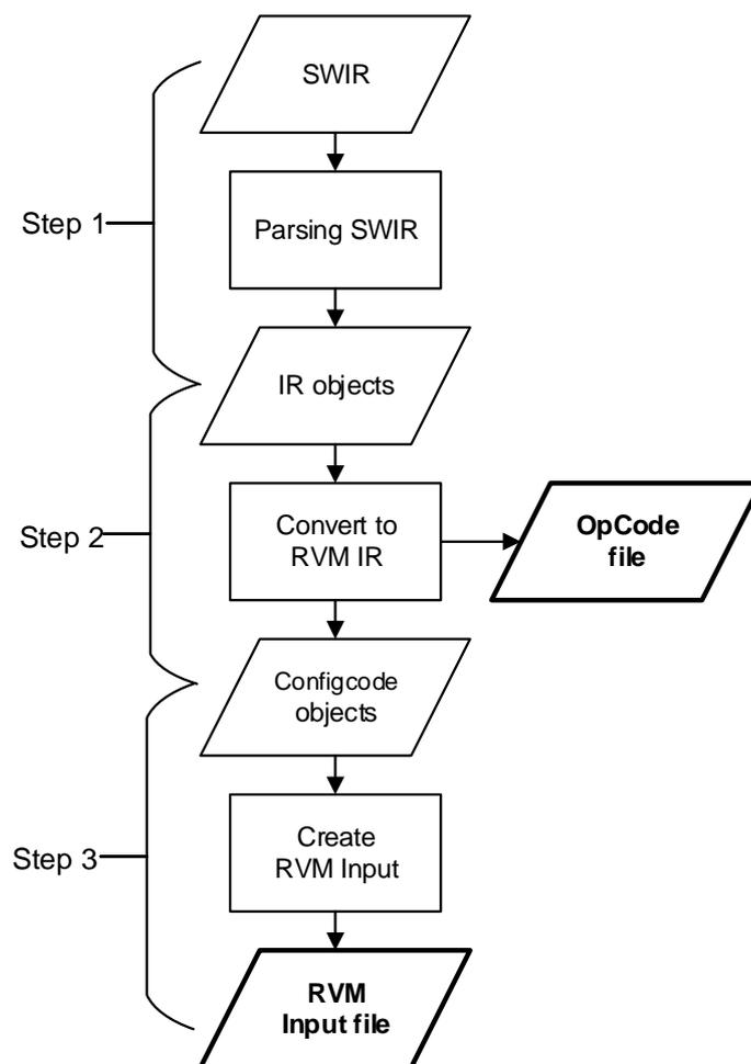
**Figure 7.1: Processing step of generating RVM Input file**
