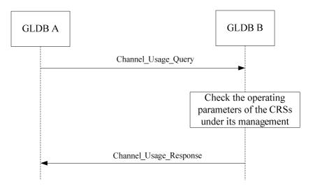
Figure 6.6: CRS operating parameters checking procedure
