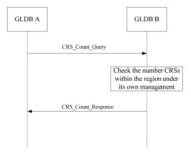
Figure 6.8: CRS number discovery procedure
