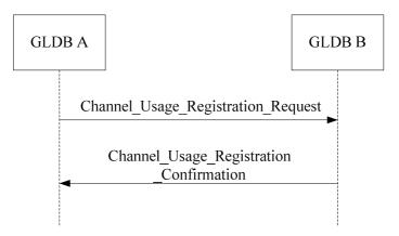
Figure 6.7: CRS channel usage registration procedure
