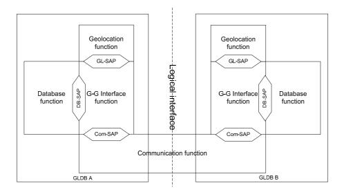
Figure 4.3: View of reference model for the information exchange between GLDBs using the G-G logical interface
