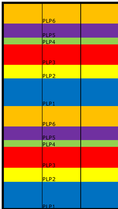
Figure 58: The matrix M_2 , showing the three rightmost columns having been moved on top of the three first columns. Each column corresponds to one RF channel (LC type D)
