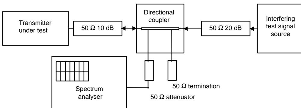
**Figure 5: Measurement arrangement**
