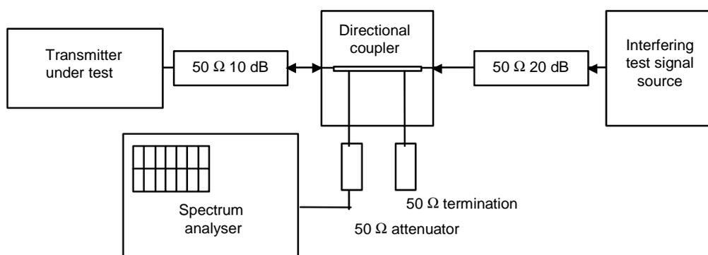
**Figure 5: Measurement arrangement**
