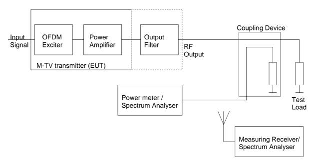
NOTE: If the transmitter does not include any output filter, an external filter shall be added after the transmitter for the testing arrangement. This filter shall be representative of the multiplexer or filter existing in operational conditions and viewed by the transmitted output when installed.
