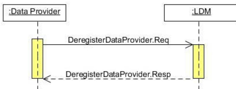
Figure 6: LDM Data Provider deregistration message sequence
