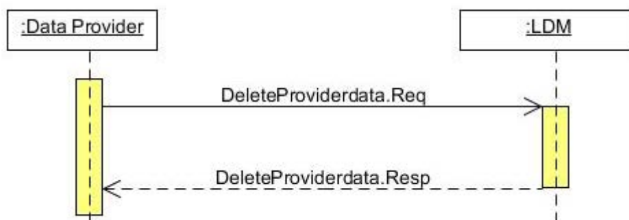
Figure 10: Delete provider data message sequence
