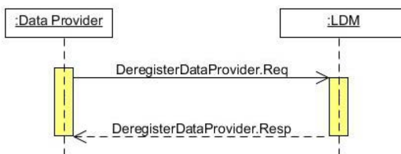
Figure 6: LDM Data Provider deregistration message sequence
