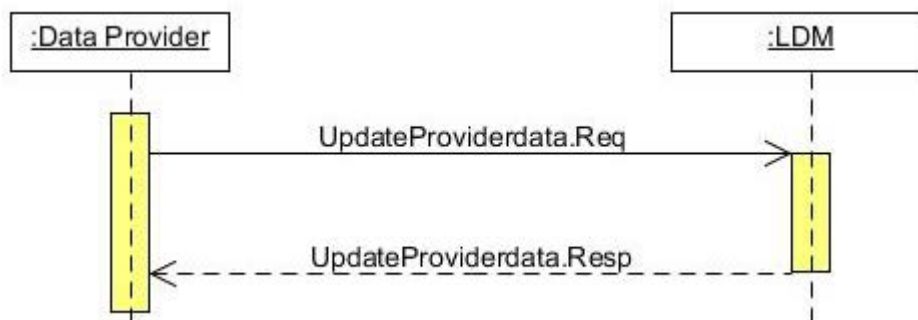
Figure 9: Update provider data message sequence
