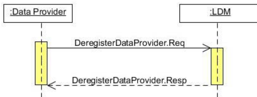
Figure 6: LDM Data Provider deregistration message sequence
