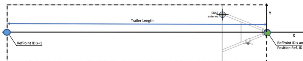
Figure 13: 4 or more wheeled larger trailer reference position
